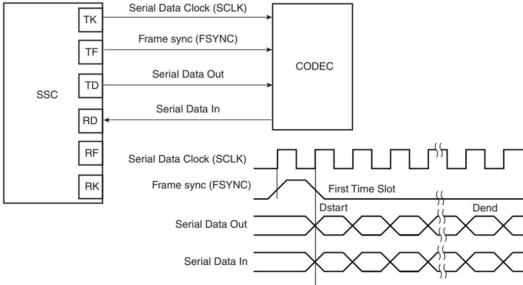
**Figure 34-19.** Time Slot Application Block Diagram
