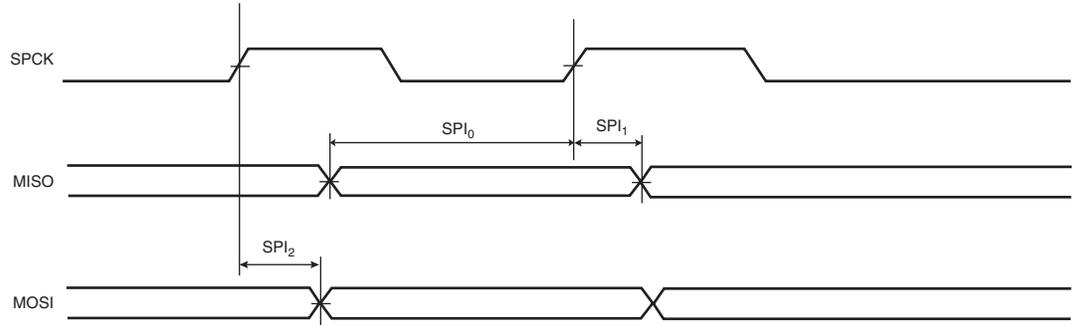
**Figure 46-8.** SPI Master Mode with (CPOL=0 and NCPHA=1) or (CPOL=1 and NCPHA=0)
