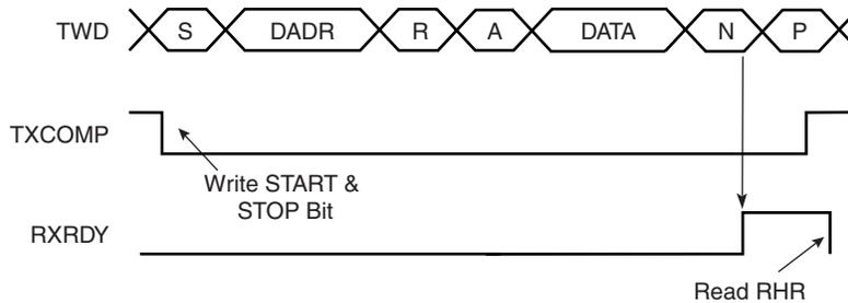
**Figure 32-9.** Master Read with Multiple Data Bytes
