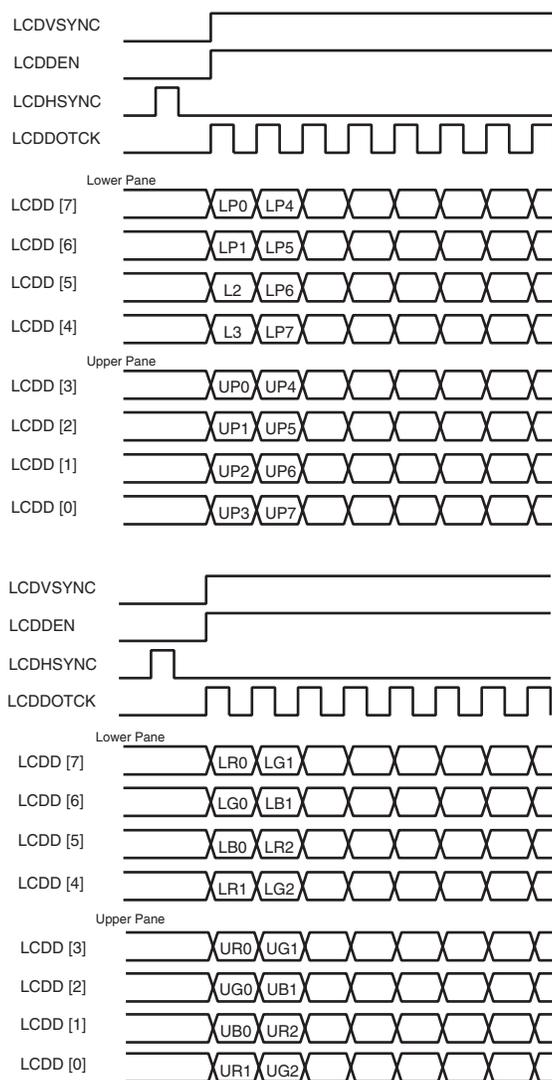
**Figure 43-10. Dual Scan Monochrome and Color 16-bit Panel Timing (First Line Expanded View)**
