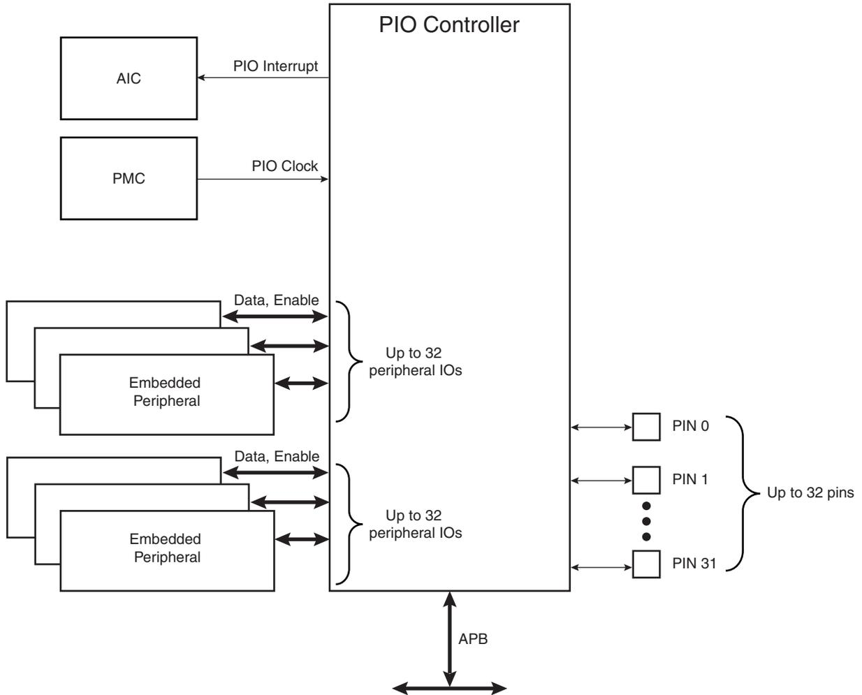
Figure 30-2. Application Block Diagram
