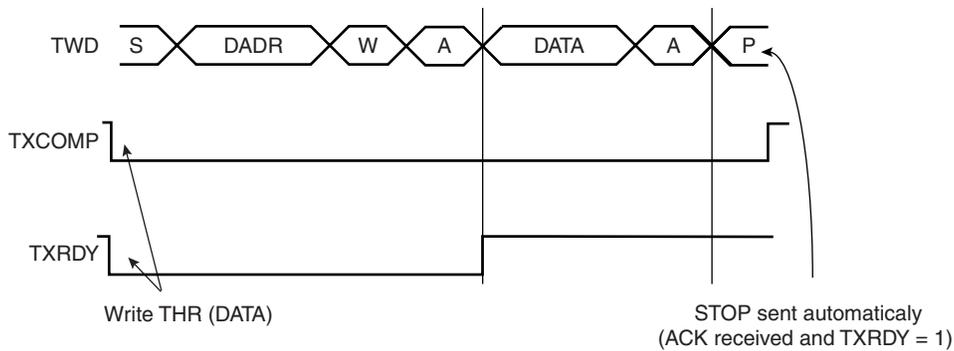
**Figure 32-6.** Master Write with Multiple Data Byte
