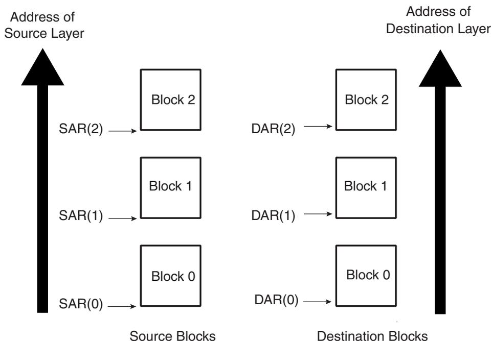
If the user needs to execute a DMA transfer where the source and destination address are contiguous but the amount of data to be transferred is greater than the maximum block size `DMAC_CTLx.BLOCK_TS`, then this can be achieved using the type of multi-block transfer as shown in [Figure 24-7 on page 285](#).
