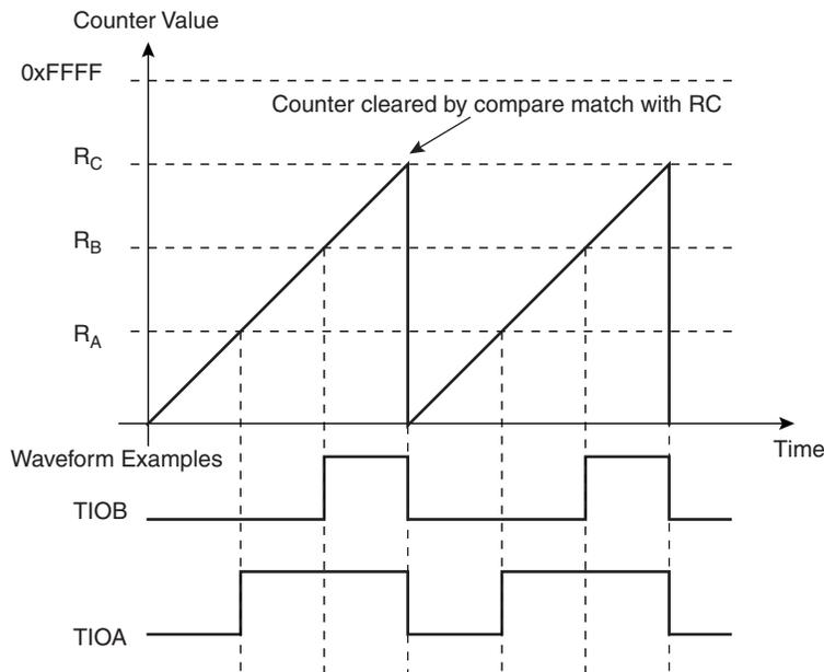
**Figure 36-10. WAVSEL = 10 With Trigger**
