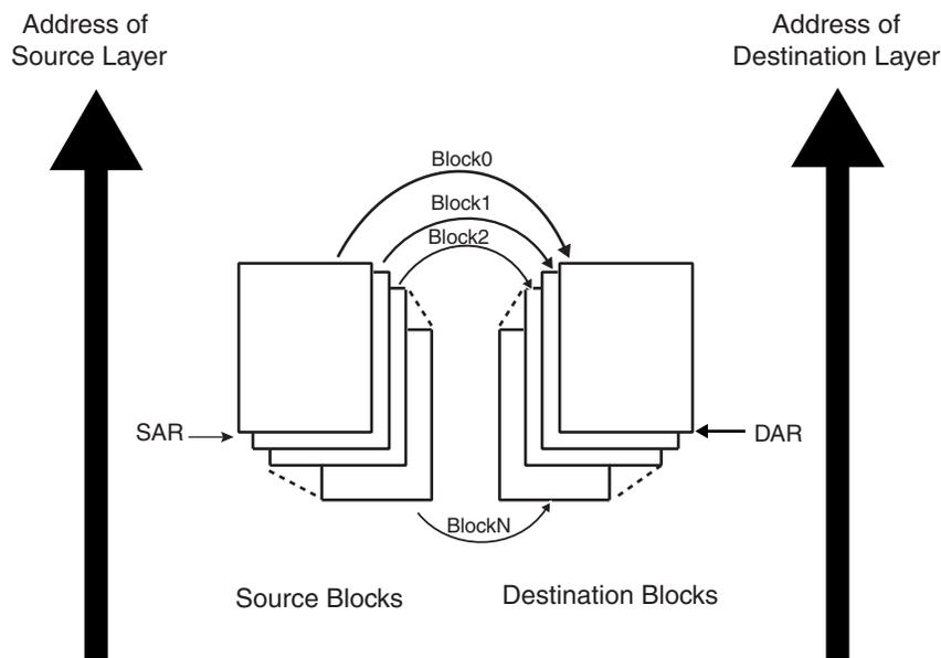
**Figure 24-10.** DMA Transfer Flow for Source and Destination Address Auto-reloaded
