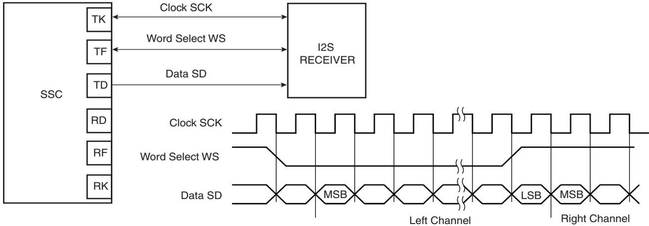
**Figure 34-18.** Codec Application Block Diagram
