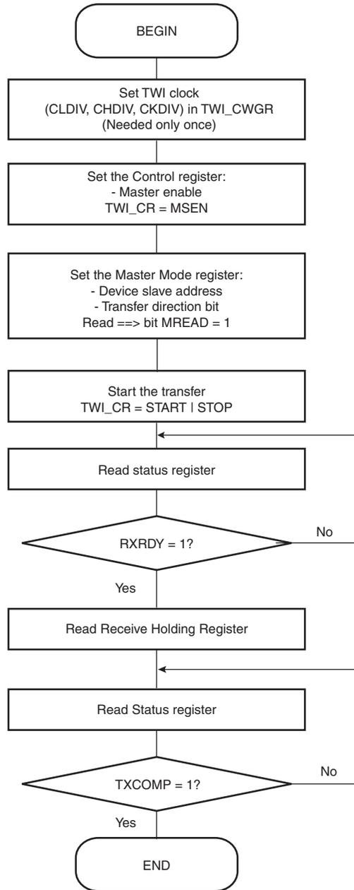
**Figure 32-17. TWI Read Operation with Single Data Byte and Internal Address**
