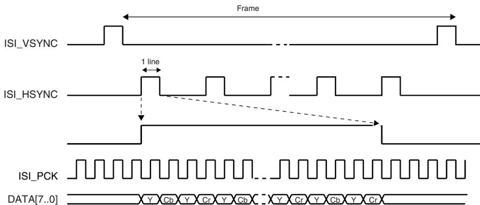
**Figure 45-4.** SAV and EAV Sequence Synchronization
