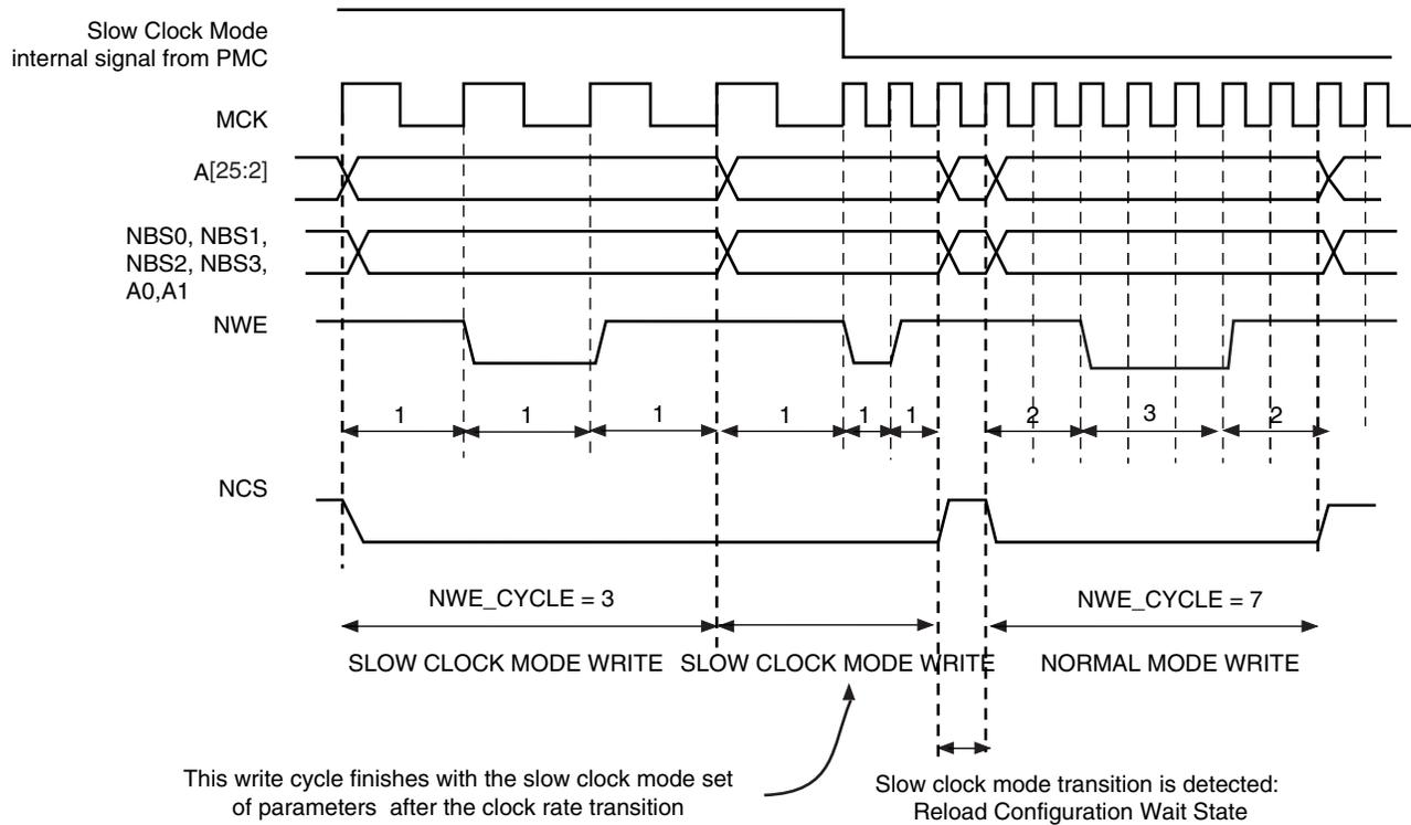
**Figure 21-33.** Recommended Procedure to Switch from Slow Clock Mode to Normal Mode or from Normal Mode to Slow Clock Mode
