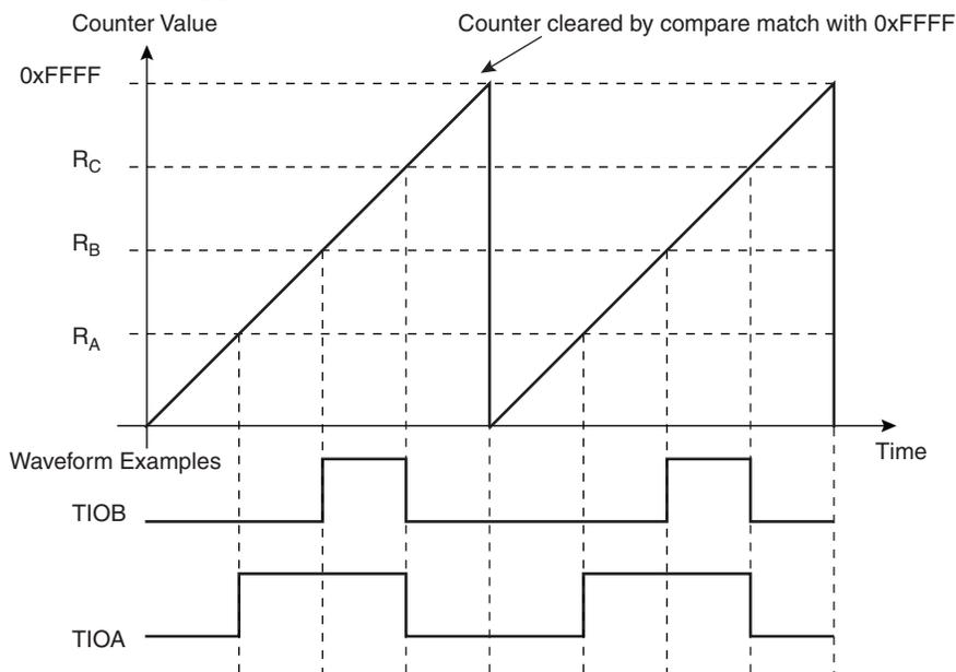
**Figure 36-8.** WAVSEL= 00 with trigger
