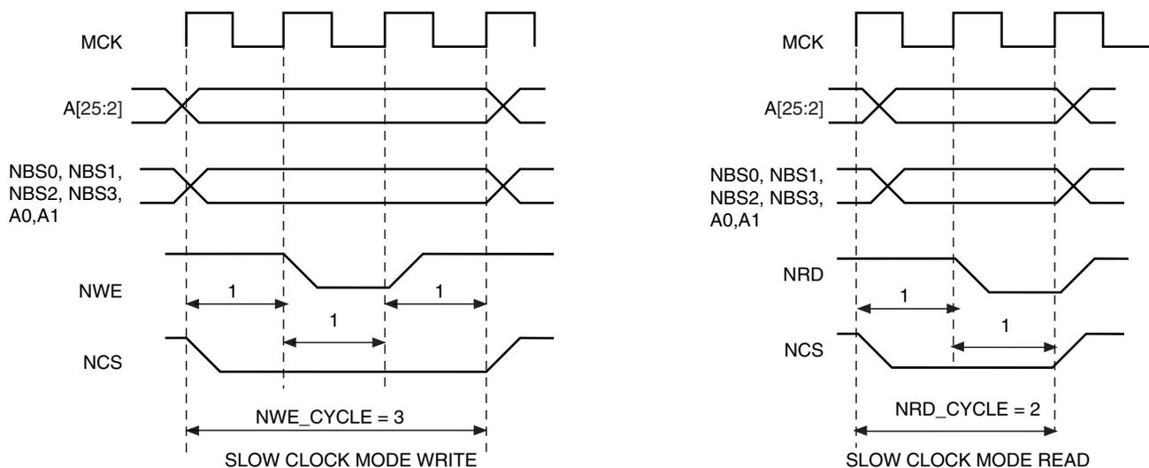
Table 21-6. Read and Write Timing Parameters in Slow Clock Mode
