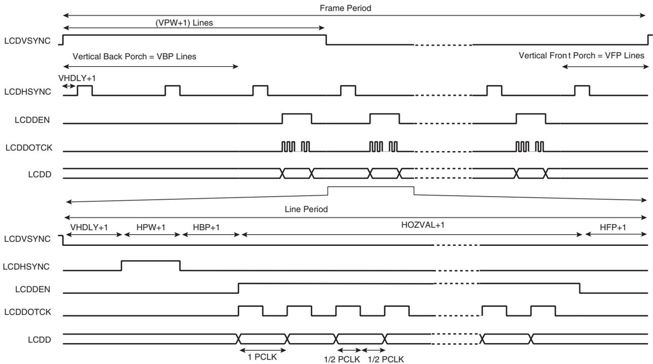
**Figure 43-5.** TFT Panel Timing (Line Expanded View), CLKMOD=1
