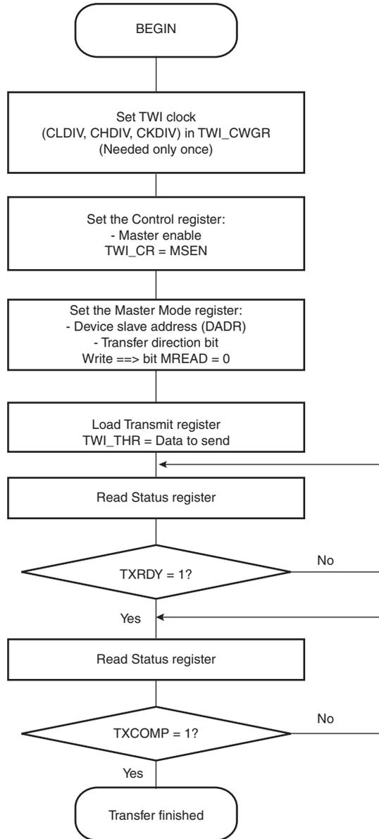
**Figure 32-14. TWI Write Operation with Single Data Byte and Internal Address**
