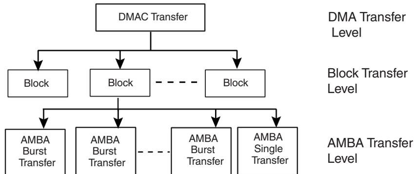
**Block:** A block of DMAC data. The amount of data (block length) is determined by the flow controller. For transfers between the DMAC and memory, a block is broken directly into a sequence of AMBA bursts and AMBA single transfers. For transfers between the DMAC and a non-memory peripheral, a block is broken into a sequence of DMAC transactions (single and bursts). These are in turn broken into a sequence of AMBA transfers.
