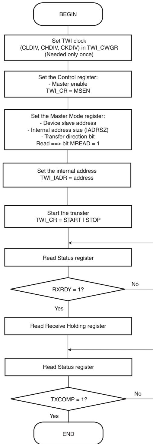
**Figure 32-18. TWI Read Operation with Multiple Data Bytes with or without Internal Address**
