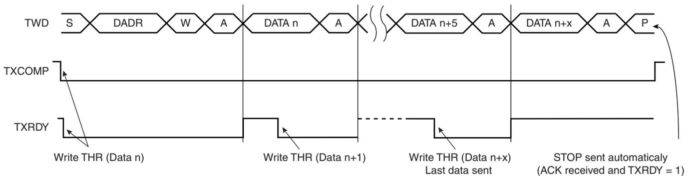
**Figure 32-7.** Master Write with One Byte Internal Address and Multiple Data Bytes
