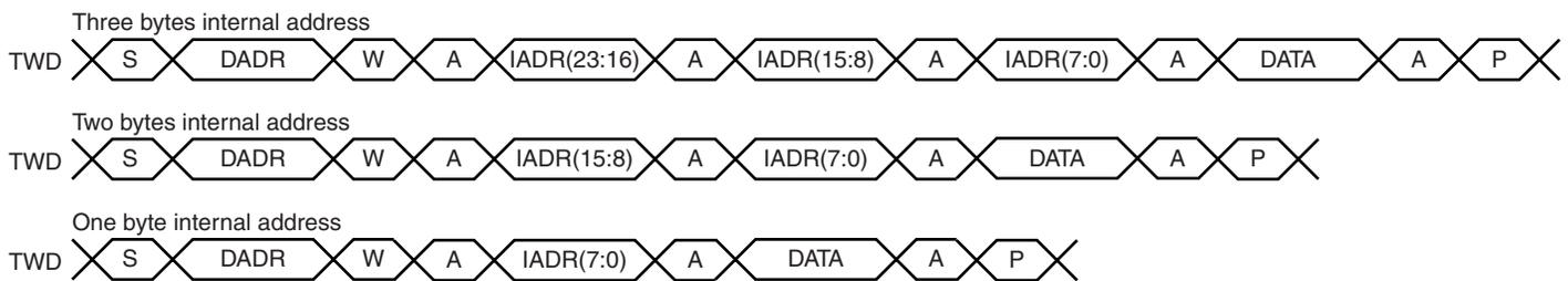
**Figure 32-11. Master Read with One, Two or Three Bytes Internal Address and One Data Byte**
