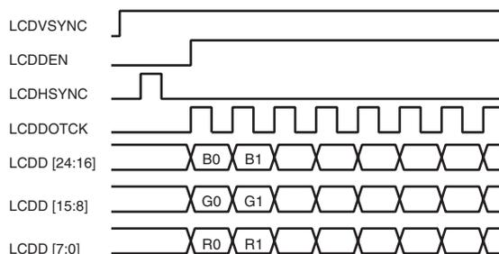
**Figure 43-7.** Single Scan Monochrome and Color 4-bit Panel Timing (First Line Expanded View)
