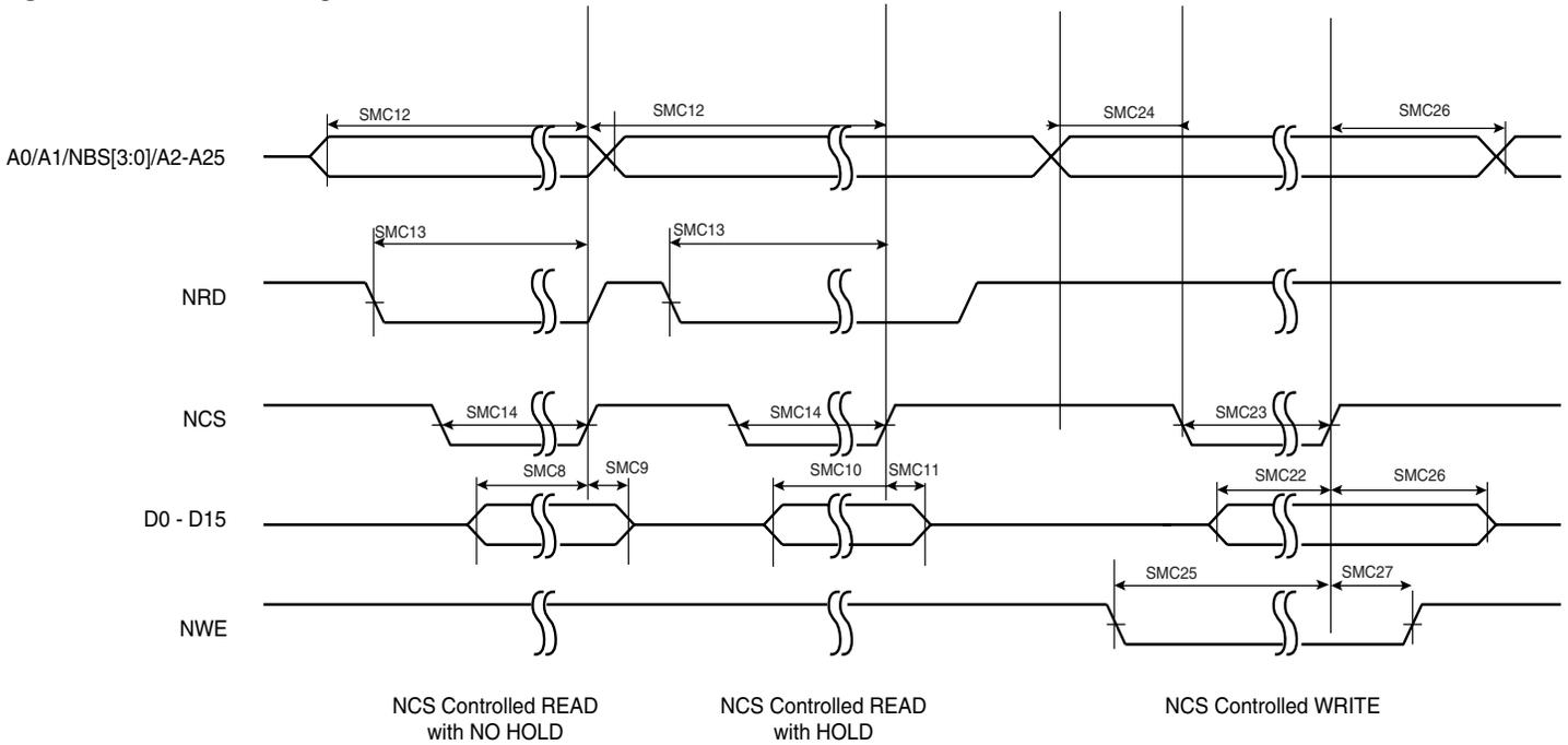
**Figure 46-3.** SMC timings - NRD controlled Read and NWE controlled Write
