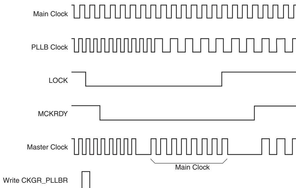
**Figure 27-7.** Programmable Clock Output Programming
