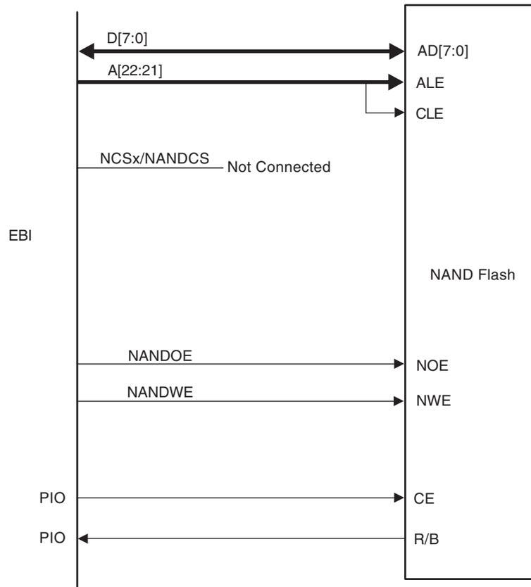
Note: The External Bus Interfaces 0 and 1 are also able to support 16-bit devices.
