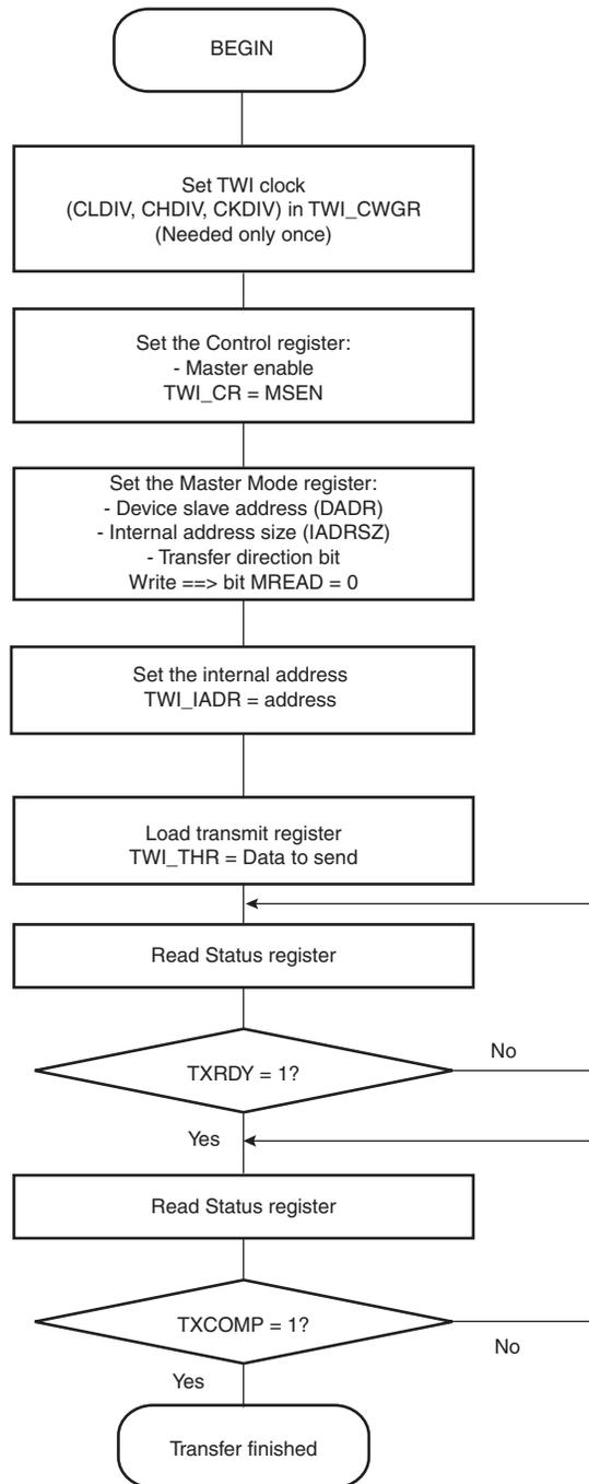
**Figure 32-15. TWI Write Operation with Multiple Data Bytes with or without Internal Address**
