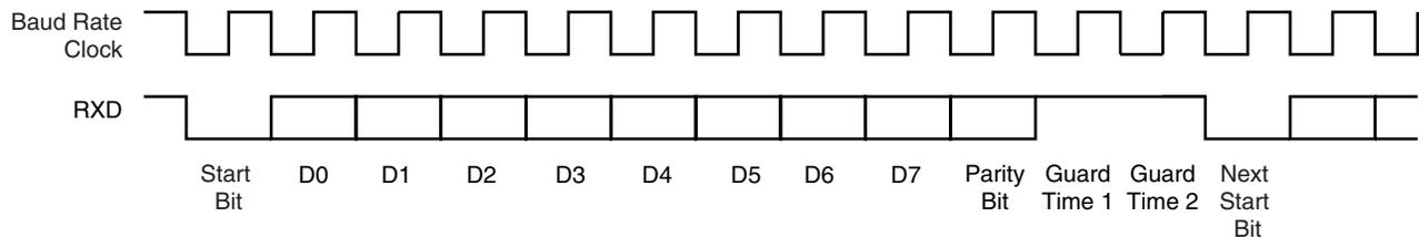
**Figure 33-22.** T = 0 Protocol with Parity Error
