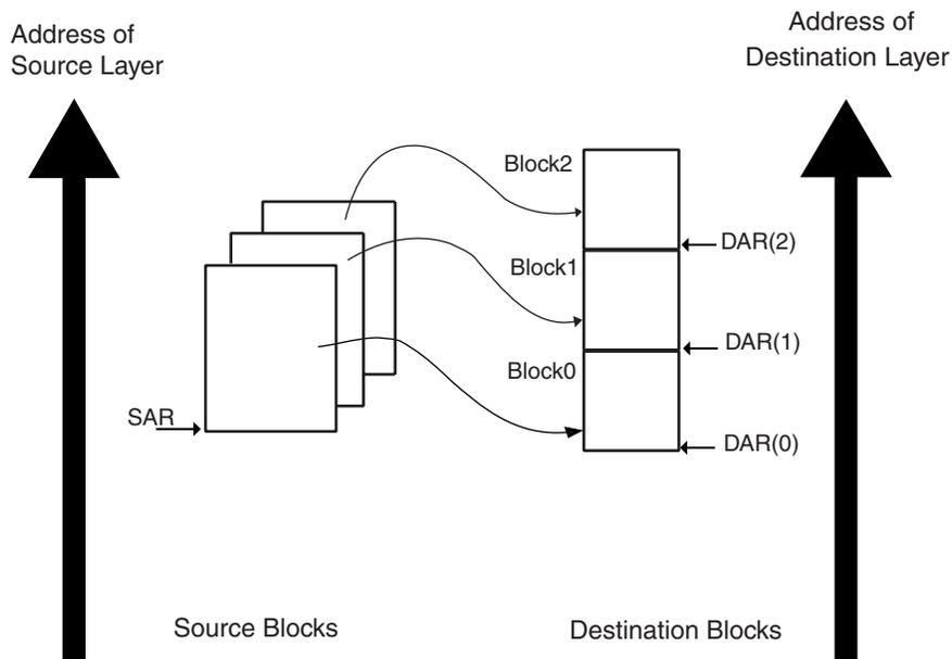
**Figure 24-14.** DMA Transfer for Source Address Auto-reloaded and Contiguous Destination Address
