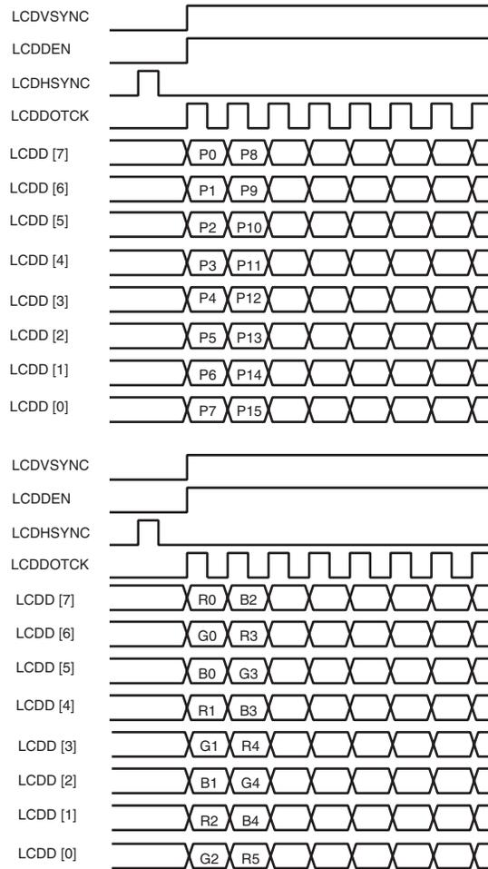
**Figure 43-9.** Dual Scan Monochrome and Color 8-bit Panel Timing (First Line Expanded View)
