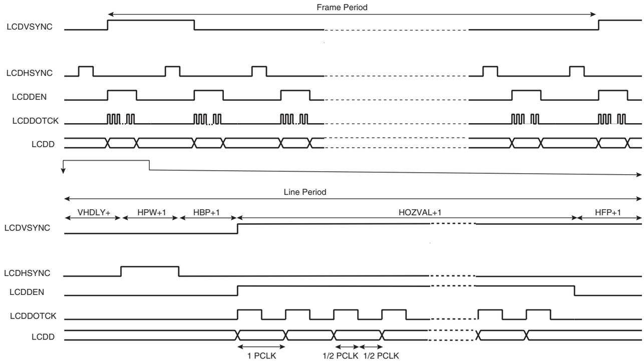
**Figure 43-4.** TFT Panel Timing, CLKMOD = 0, VPW = 2, VBP = 2, VFP = 1
