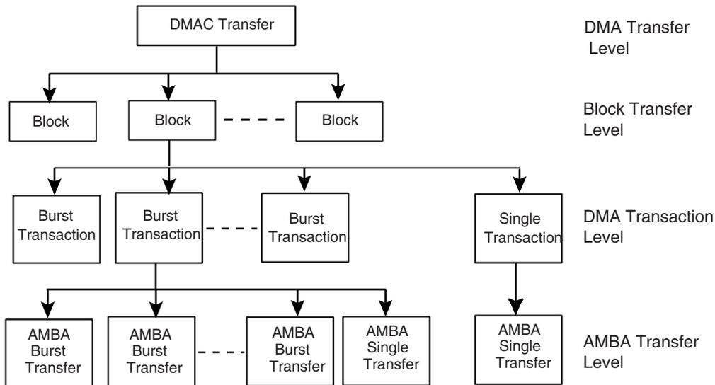
**Figure 24-3.** DMAC Transfer Hierarchy for Memory
