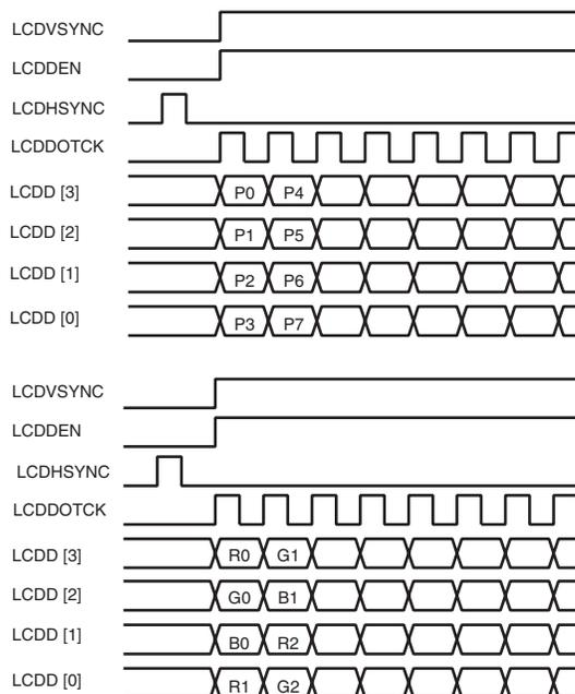
**Figure 43-8. Single Scan Monochrome and Color 8-bit Panel Timing (First Line Expanded View)**
