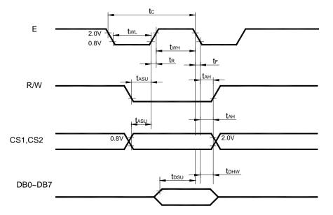
Figure 5.0 MPU write timing
