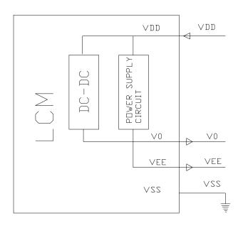
$VDD-V0(V_{LCD})$ :LCD Driving voltage
