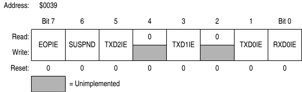
Figure 9-16. USB Interrupt Register 0 (UIR0)
