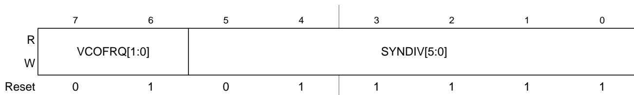
Figure 7-4. S12CPMU Synthesizer Register (CPMUSYNR)
