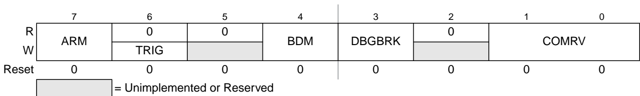
Figure 6-3. Debug Control Register (DBGC1)
