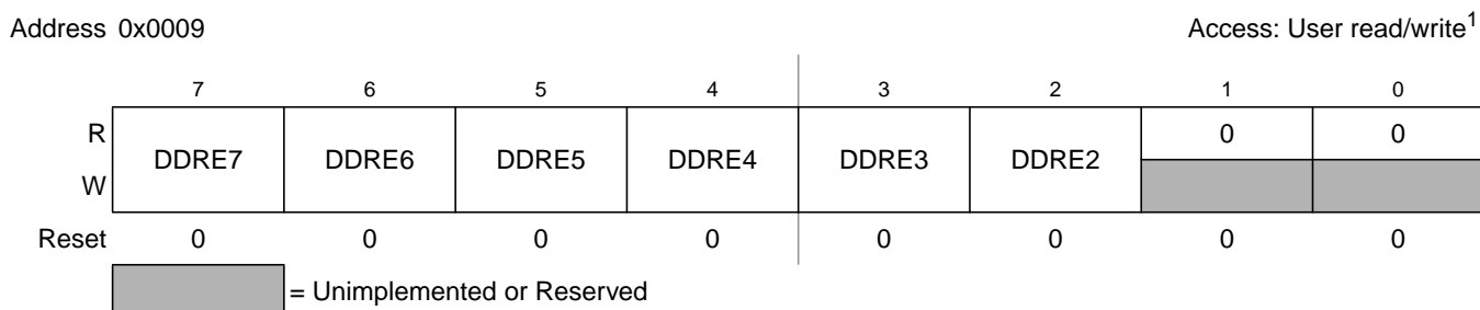
Figure 2-7. Port E Data Direction Register (DDRE)
