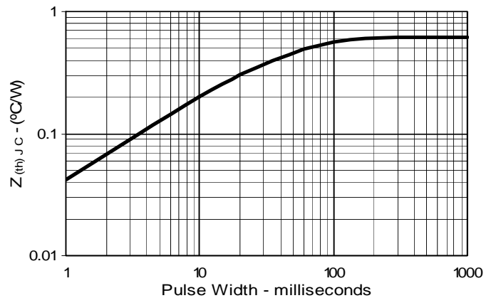
Fig. 12. Maximum Transient Thermal Impedance
