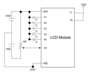
\* (T1, T2)=(H, H) \*\* VLCD (LCD Driving Voltage)=VDD-V5
