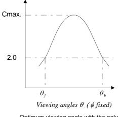
Optimum viewing angle with the naked eye and viewing angle  $\theta$  at Cmax. Above are not always the same.
