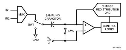
FIGURE 1. ADC122S021 in Track Mode
