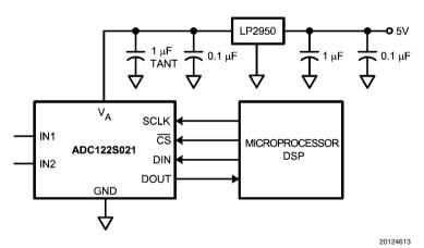
FIGURE 4. Typical Application Circuit
