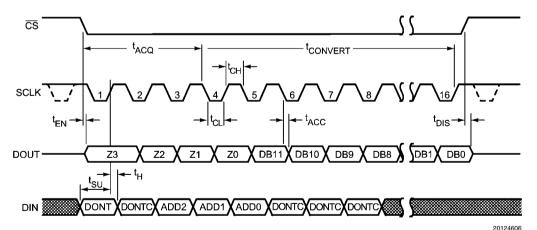
ADC122S021 Serial Timing Diagram
