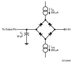
**Timing Test Circuit**
