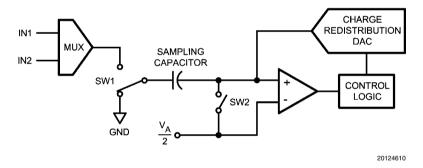
FIGURE 2. ADC122S021 in Hold Mode
