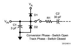
FIGURE 5. Equivalent Input Circuit
