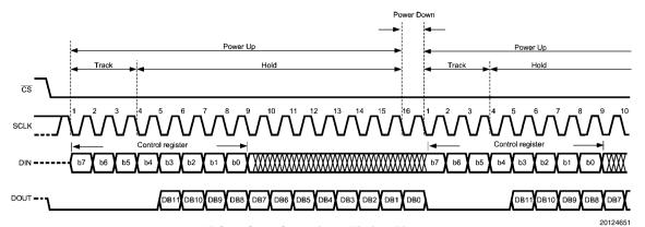
**ADC122S021 Operational Timing Diagram**
