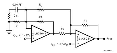
FIGURE 7. Two Op-Amp Instrumentation Amplifier
