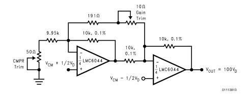
FIGURE 8. Low-Power Two-Op-Amp Instrumentation Amplifier
