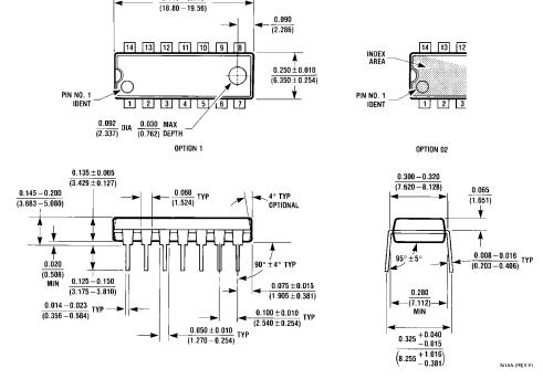
14-Pin Molded DIP Order Package Number LMC6044AIN or LMC6044IN **NS Package Number N14A**
