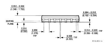
14-Pin Small Outline Order Package Number LMC6044AIM, LMC6044AIMX, LMC6044IM or LMC6044IMX NS Package Number M14A
