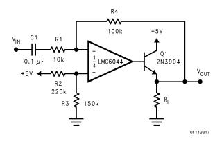
FIGURE 12. AC Coupled Power Amplifier
