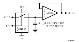
FIGURE 9. Low-Leakage Sample-and-Hold
