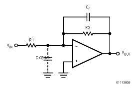
FIGURE 1. Canceling the Effect of Input Capacitance
