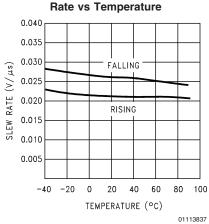
Inverting Slew Rate vs Temperature
