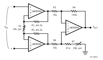
FIGURE 10. Instrumentation Amplifier
