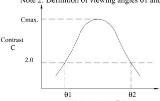
viewing angle  $\theta$  ( $\emptyset$  fixed) Optimum viewing angle with the naked eye and viewing angle  $\theta$  at Cmax. Above are not always the
