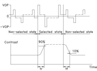
Note: Measured with a transmissive LCD panel which is displayed 1 cm<sup>2</sup>
