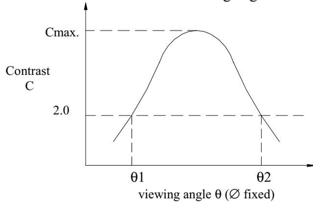
Note : Optimum viewing angle with the naked eye and viewing angle  $\theta$  at Cmax. Above are not always the same
