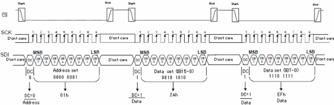
7-8. Input Data Signals and Display Position on the screen
