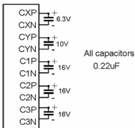
Note 3) Stabilization and charge sharing Capacitors
