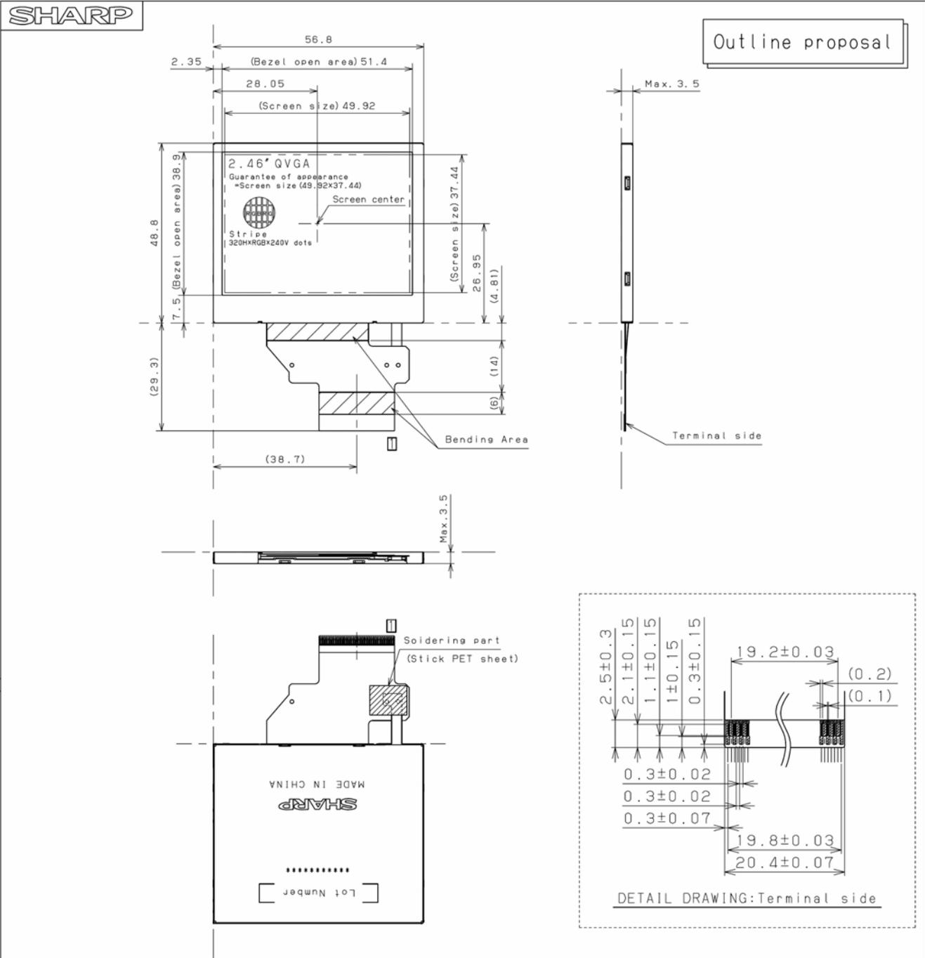
Recommended connector: FH26G (HIROSE ELECTRIC CO., LTD.) or 6281 (KYOCERA ELCO CORP.)
