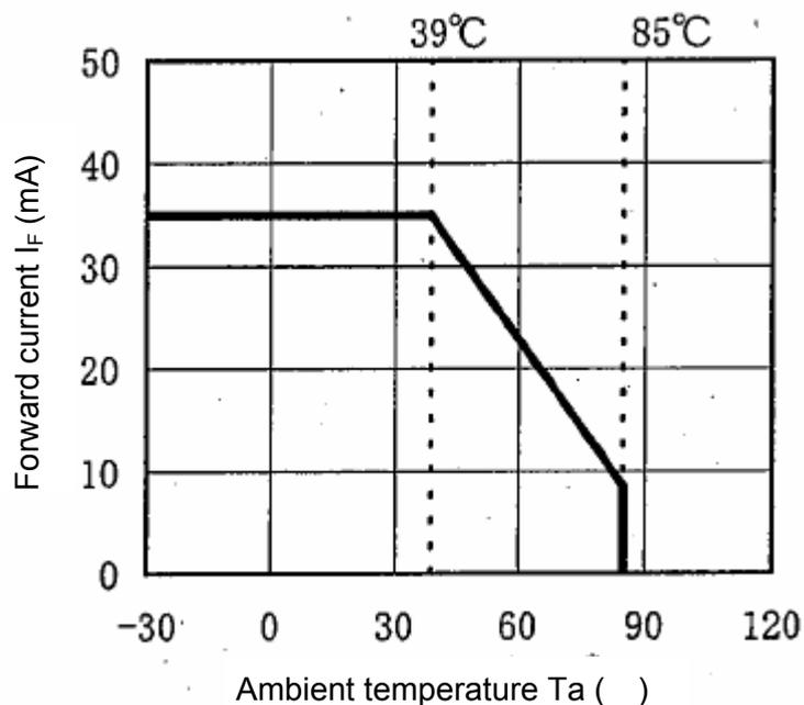
Ambient temperature of LED and the maximum input
