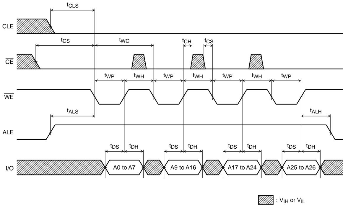
Data Input Cycle Timing Diagram
