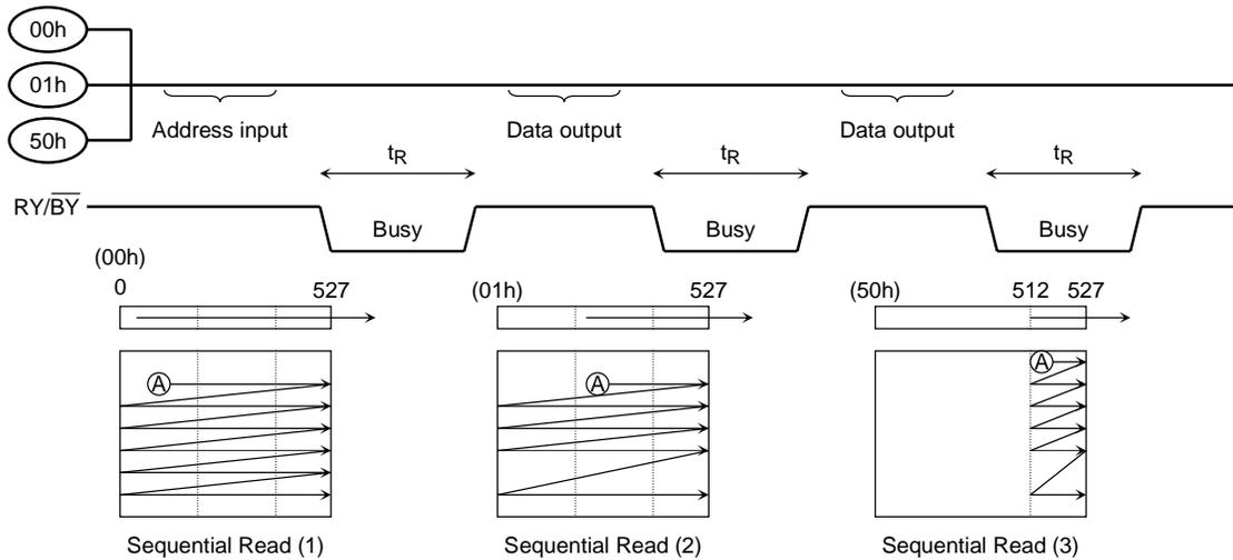
Sequential Read mode (1) and (2) output the contents of addresses 0 to 257 as shown above, while Sequential Read mode (3) outputs the contents of the redundant address locations only.
