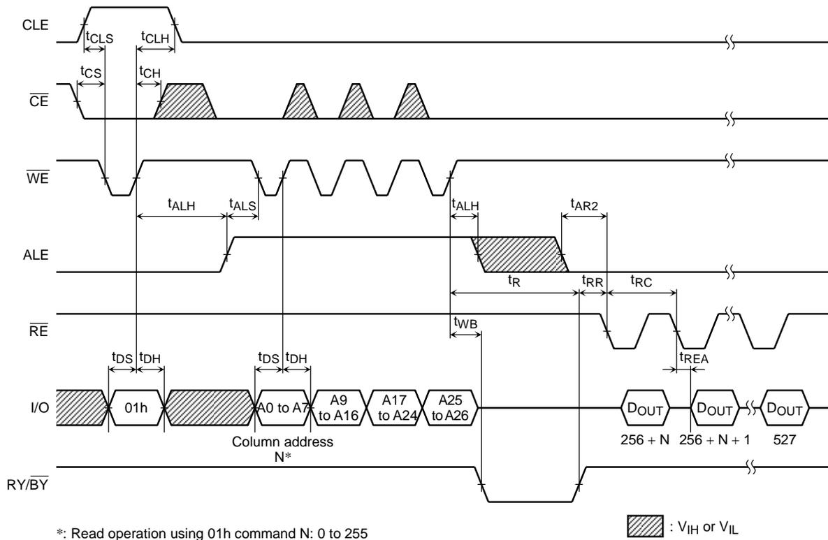
Read Cycle (3) Timing Diagram
