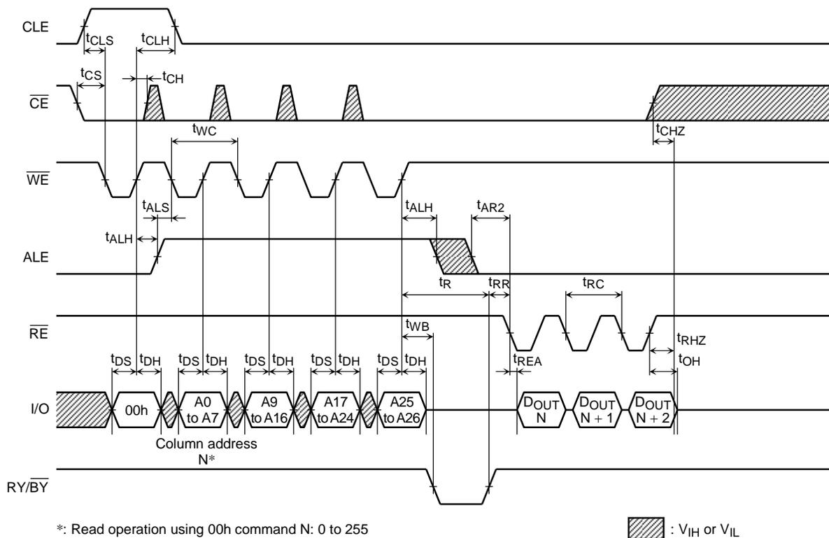
Read Cycle (2) Timing Diagram
