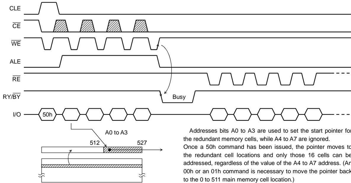
Figure 4. Read mode (3) operation
