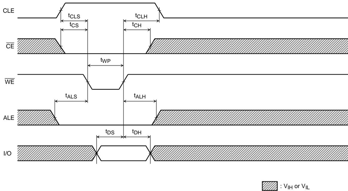
Address Input Cycle Timing Diagram
