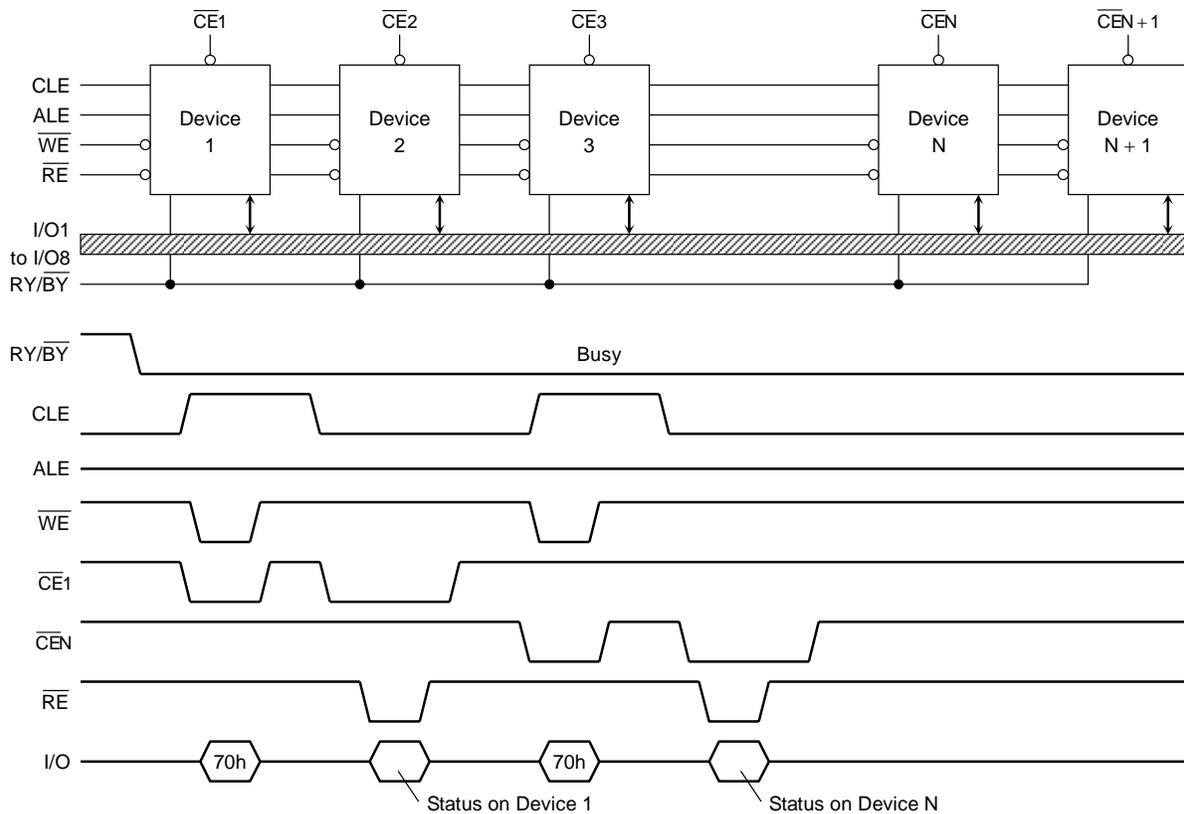
Figure 5. Status Read timing application example
