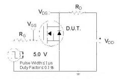
Fig 10a. Switching Time Test Circuit
