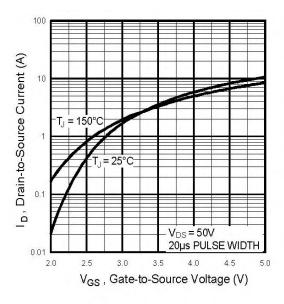
Fig 3. Typical Transfer Characteristics
