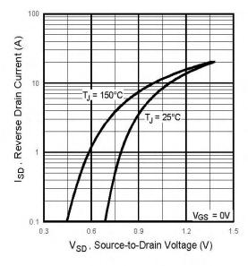
**Fig 7.** Typical Source-Drain Diode Forward Voltage
