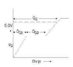
Fig 13a. Basic Gate Charge Waveform
