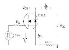
Fig 12a. Unclamped Inductive Test Circuit
