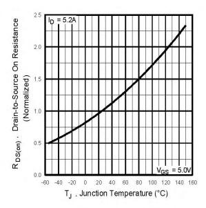
Fig 4. Normalized On-Resistance Vs. Temperature
