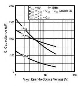
**Fig 5.** Typical Capacitance Vs. Drain-to-Source Voltage
