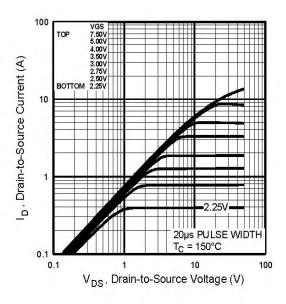
Fig 2. Typical Output Characteristics,  $T_C = 150$ °C
