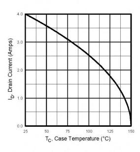
**Fig 9.** Maximum Drain Current Vs. Case Temperature
