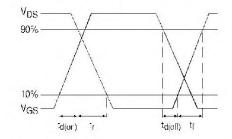
Fig 10b. Switching Time Waveforms
