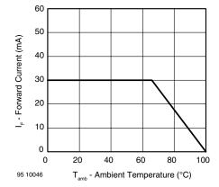
Figure 2. Forward Current vs. Ambient Temperature
