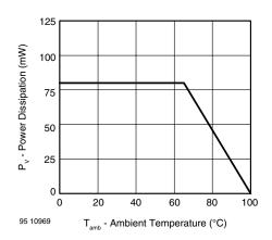
Figure 1. Power Dissipation vs. Ambient Temperature
