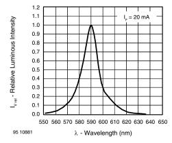
Figure 8. Relative Intensity vs. Wavelength
