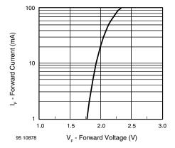
Figure 4. Forward Current vs. Forward Voltage
