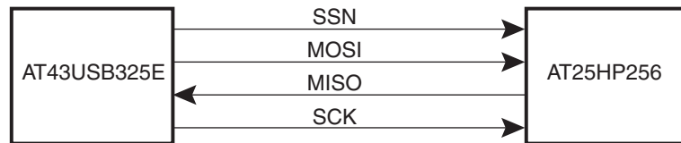
Figure 3. AT43USB325E Read Sequence
