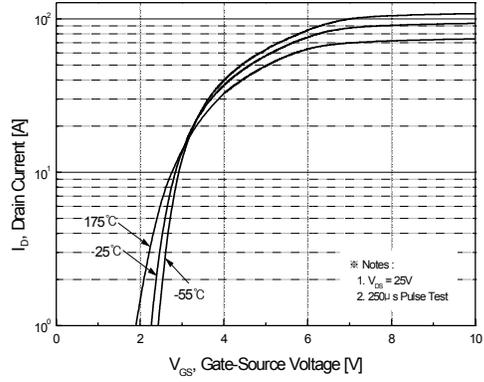
**Figure 2. Transfer Characteristics**
