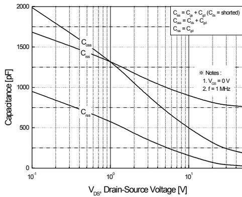
**Figure 5. Capacitance Characteristics**
