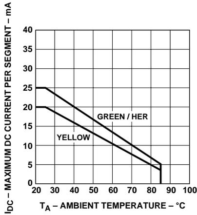
Figure 1. Maximum allowable DC current vs. ambient temperature.
