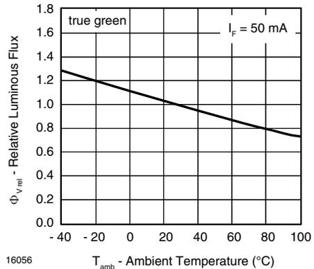
Figure 6. Rel. Luminous Flux vs. Ambient Temperature
