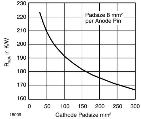
Figure 4. Thermal Resistance Junction Ambient vs. Cathode Padsize
