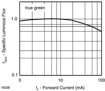
Figure 7. Specific Luminous Flux vs. Forward Current
