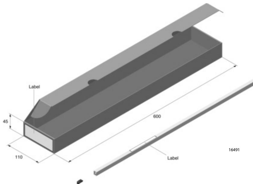
**TUBE WITH BAR CODE LABEL** Dimensions in millimeters
