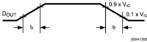
FIGURE 3. D_{OUT} Rise and Fall Times
