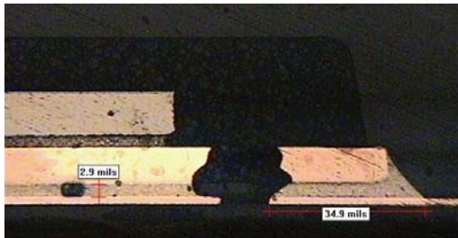
50% Paste Coverage, Plugged Via, 2.9 mil Standoff
