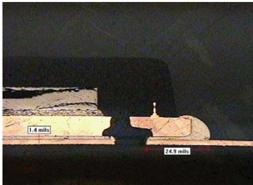
37% Paste Coverage, Plugged Via, 1.4 mil Standoff
