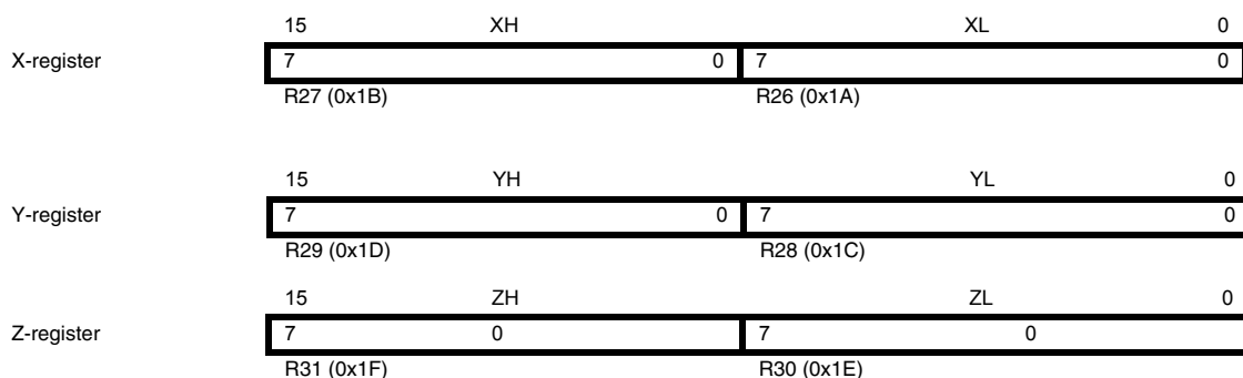
Figure 6-3. The X-, Y-, and Z-registers
