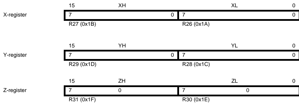
Figure 7-3. The X-, Y-, and Z-registers
