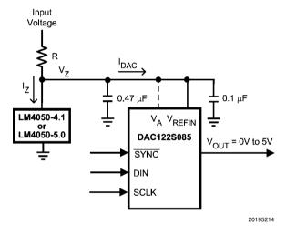
FIGURE 6. The LM4050 as a power supply
