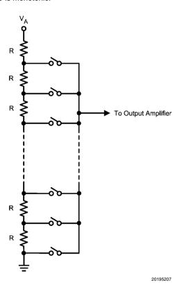
FIGURE 3. DAC Resistor String
