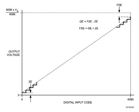
FIGURE 1. Input / Output Transfer Characteristic
