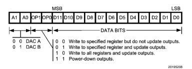
**FIGURE 4. Input Register Contents**
