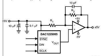
FIGURE 9. Bipolar Operation
