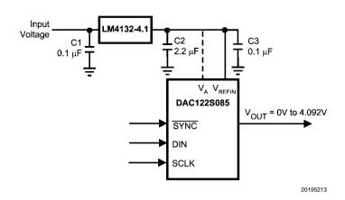
FIGURE 5. The LM4130 as a power supply
