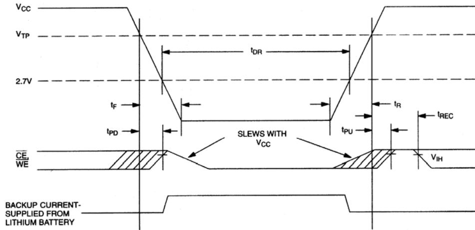
**POWER-DOWN/POWER-UP TIMING**(t<sub>A</sub>: See Note 10)
