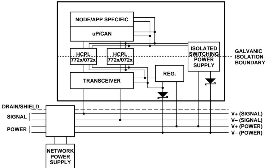
Figure 18. Isolated node powered by the network.
