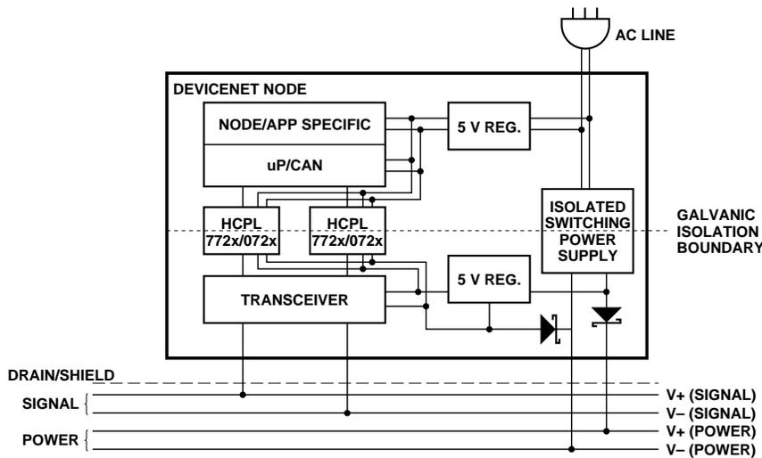
Figure 20. Isolated node providing power to the network.
