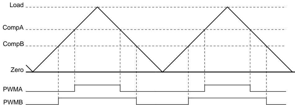
In this example, the first generator is set to drive High on match A up, drive Low on match A down, and ignore the other four events. The second generator is set to drive High on match B up, drive Low on match B down, and ignore the other four events. Changing the value of comparator A changes the duty cycle of the  $PWMA$  signal, and changing the value of comparator B changes the duty cycle of the  $PWMB$  signal.
