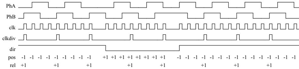
The period of the timer is configurable by specifying the load value for the timer in the **QEILOAD** register. When the timer reaches zero, an interrupt can be triggered, and the hardware reloads the timer with the **QEILOAD** value and continues to count down. At lower encoder speeds, a longer timer period is needed to be able to capture enough edges to have a meaningful result. At higher encoder speeds, both a shorter timer period and/or the velocity predivider can be used.
