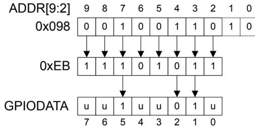
During a read, if the address bit associated with the data bit is set to 1, the value is read. If the address bit associated with the data bit is set to 0, it is read as a zero, regardless of its actual value. For example, reading address GPIODATA + 0x0C4 yields as shown in Figure 9-3 on page 166.
