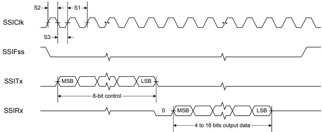
Figure 21-6. SSI Timing for SPI Frame Format (FRF=00), with SPH=1
