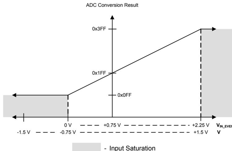
Figure 11-4. Differential Sampling Range,  $V_{IN\_ODD} = 2.25\text{ V}$
