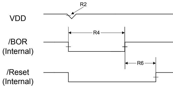
**Figure 20-12. Software Reset Timing**
