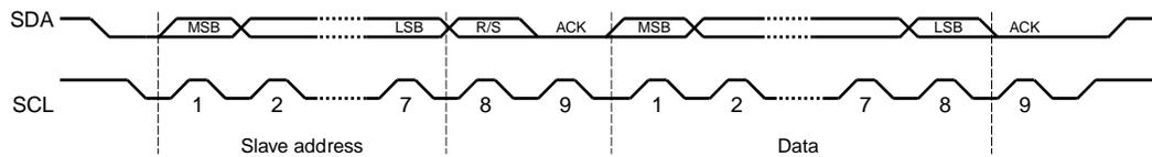
The first seven bits of the first byte make up the slave address (see Figure 14-5 on page 354). The eighth bit determines the direction of the message. A zero in the R/S position of the first byte means that the master will write (send) data to the selected slave, and a one in this position means that the master will receive data from the slave.
