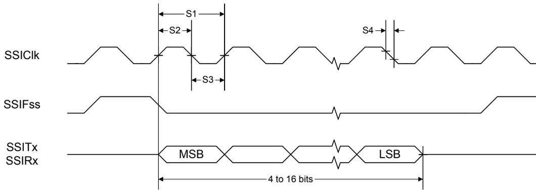
Figure 23-5. SSI Timing for MICROWIRE Frame Format (FRF=10), Single Transfer
