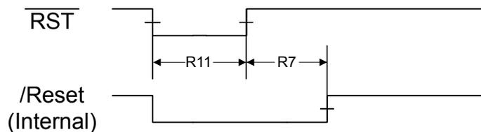
**Figure 23-11. Power-On Reset Timing**
