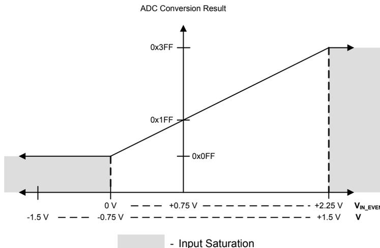
Figure 12-4. Differential Sampling Range,  $V_{IN\_ODD} = 2.25\text{ V}$
