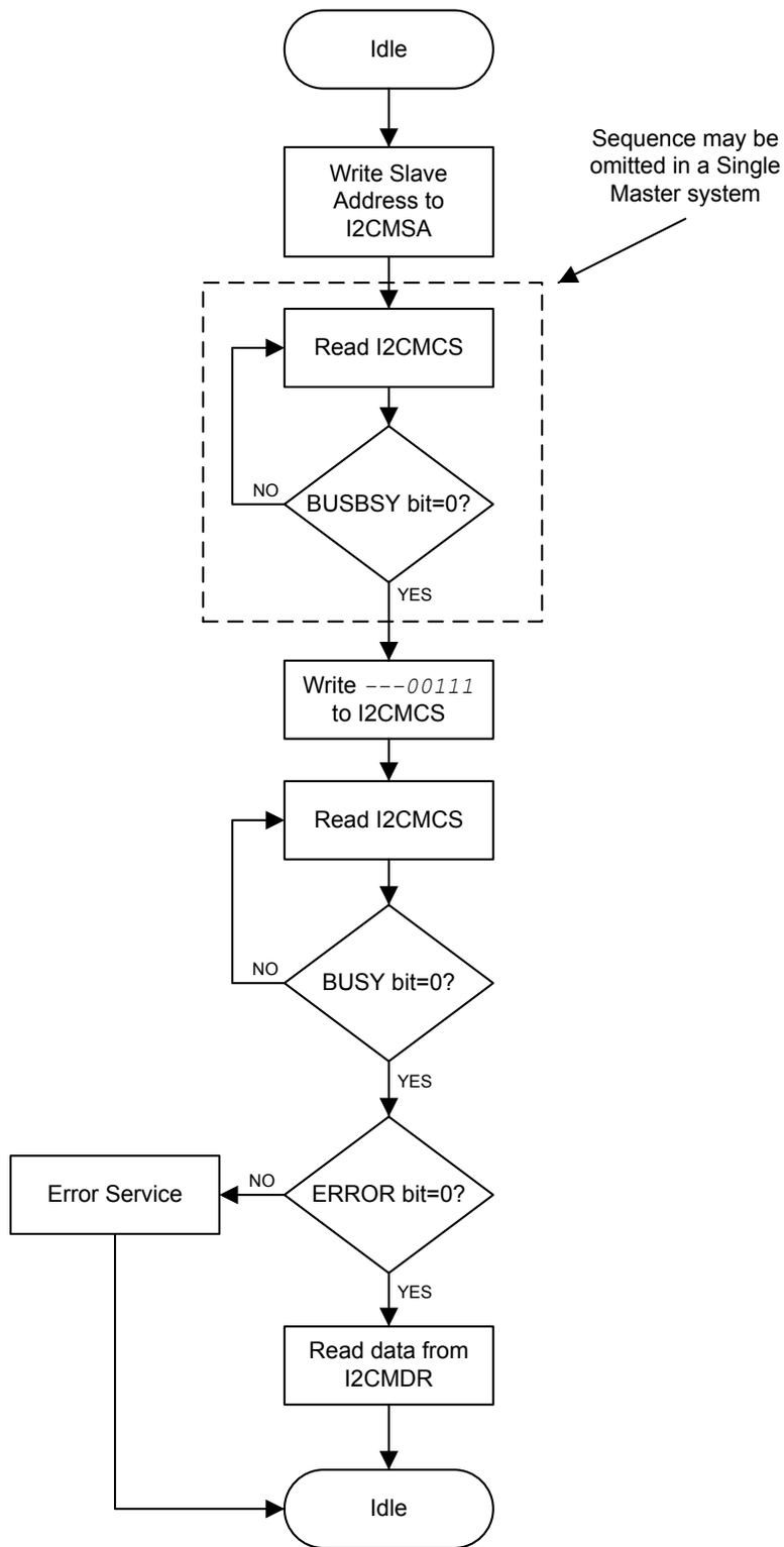
Figure 16-9. Master TRANSMIT with Repeated START
