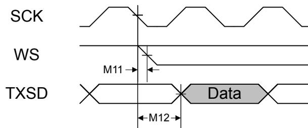
**Figure 26-18. I<sup>2</sup>S Master Mode Receive Timing**
