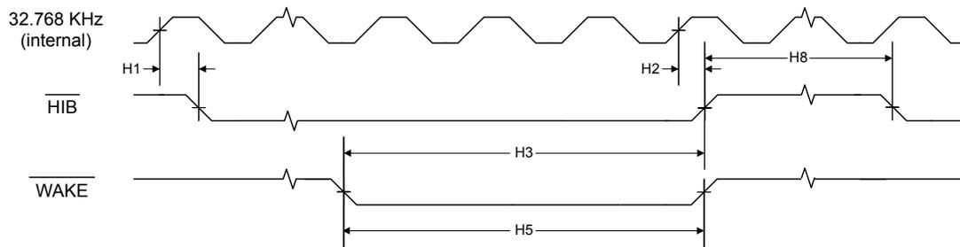
**Figure 26-11. Hibernation Module Timing with Internal Oscillator Stopped in Hibernation**
