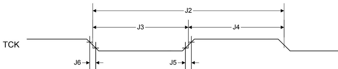
Figure 26-3. JTAG Test Access Port (TAP) Timing
