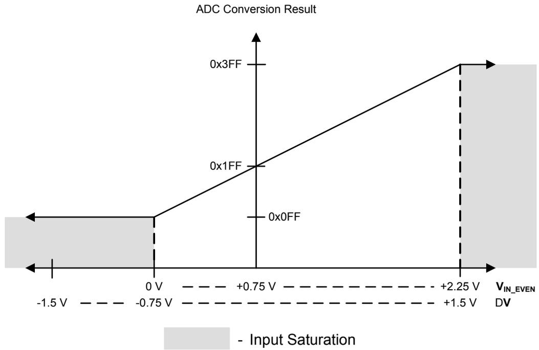
Figure 13-7. Differential Sampling Range,  $V_{IN\_ODD} = 2.25\text{ V}$
