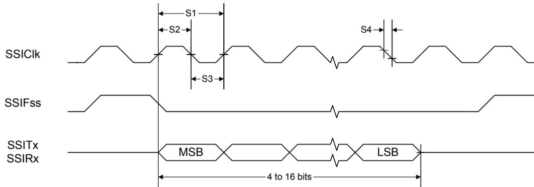
Figure 22-6. SSI Timing for MICROWIRE Frame Format (FRF=10), Single Transfer
