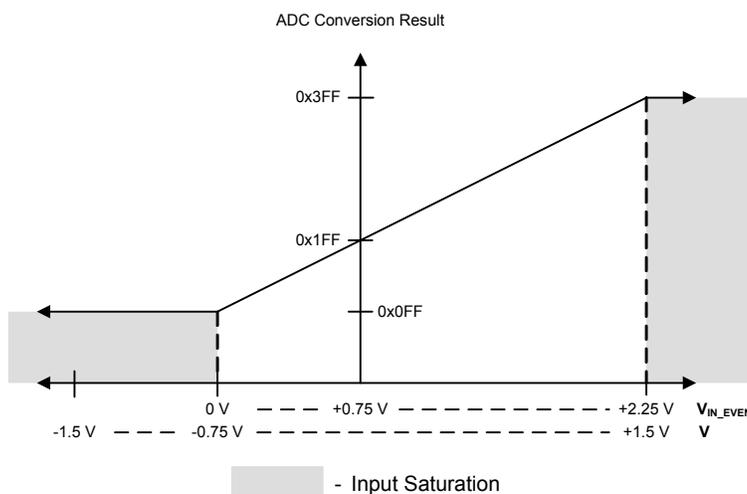
Figure 12-4. Differential Sampling Range,  $V_{IN\_ODD} = 2.25\text{ V}$
