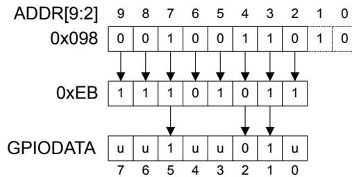
During a read, if the address bit associated with the data bit is set to 1, the value is read. If the address bit associated with the data bit is set to 0, it is read as a zero, regardless of its actual value. For example, reading address GPIODATA + 0x0C4 yields as shown in Figure 9-3 on page 171.
