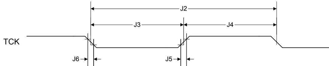
Figure 22-9. JTAG Test Access Port (TAP) Timing
