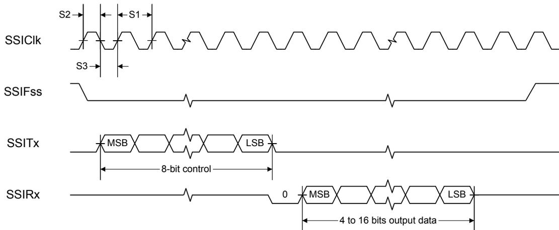
Figure 22-7. SSI Timing for SPI Frame Format (FRF=00), with SPH=1
