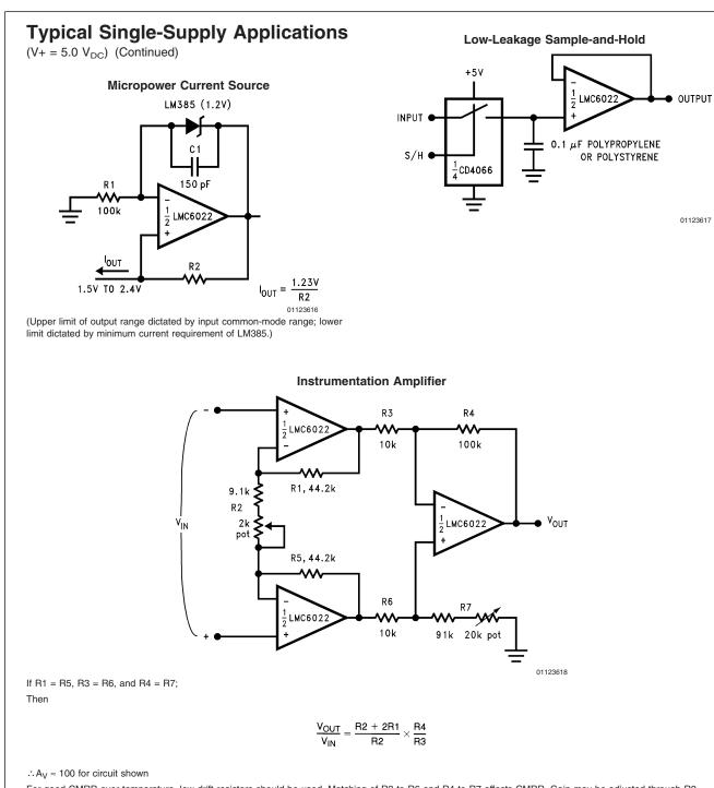
For good CMRR over temperature, low drift resistors should be used. Matching of R3 to R6 and R4 to R7 affects CMRR. Gain may be adjusted through R2. CMRR may be adjusted through R7.
