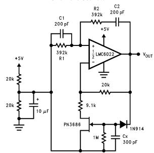
Oscillator frequency is determined by R1, R2, C1, and C2:  $f_{OSC} = 1/2\pi RC$ where R = R1 = R2 and C = C1 = C2.
