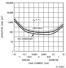
Note: Avoid resistive loads of less than  $500\Omega$ , as they may cause instability.
