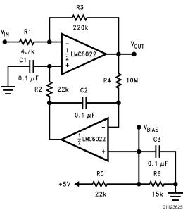
Output offset voltage reduced to the level of the input offset voltage of the bottom amplifier (typically 1 mV), referred to V<sub>BIAS</sub>.
