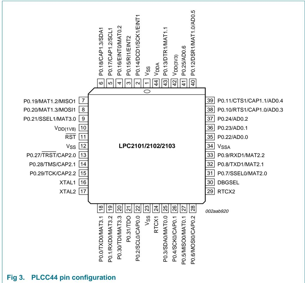
Fig 3. PLCC44 pin configuration
