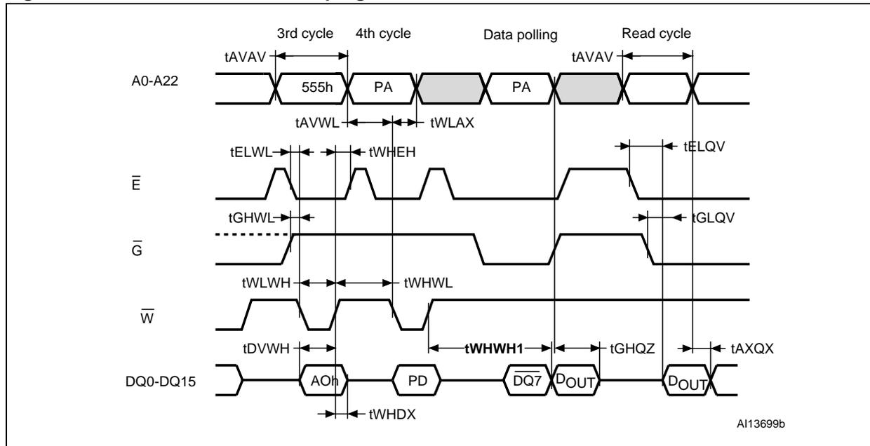
1. Only the third and fourth cycles of the Program command are represented. The Program command is followed by the check of status register data polling bit and by a read operation that outputs the data, DOUT, programmed by the previous Program command.
