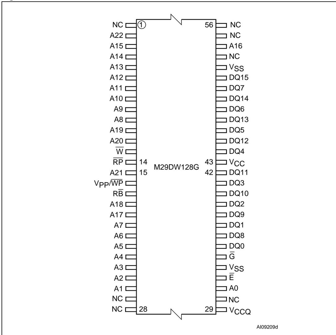
Figure 3. TBGA connections (top view through package)
