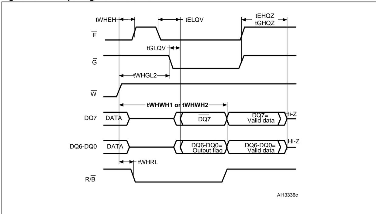
1. DQ7 returns valid data bit when the ongoing Program or Erase command is completed.
