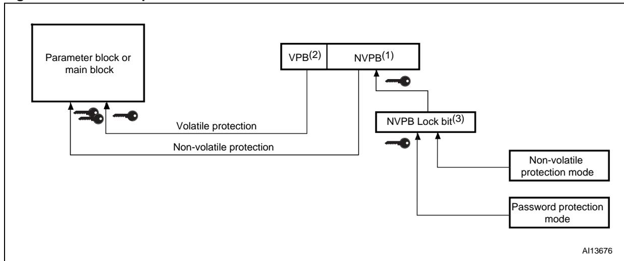
1. NVPBs default to '1' (block unprotected) after power-up and hardware reset. A block is protected or unprotected when its NVPB is set to '0' and '1', respectively. NVPBs are programmed individually and cleared collectively.
