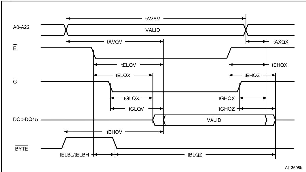
Figure 14. Page read AC waveforms
