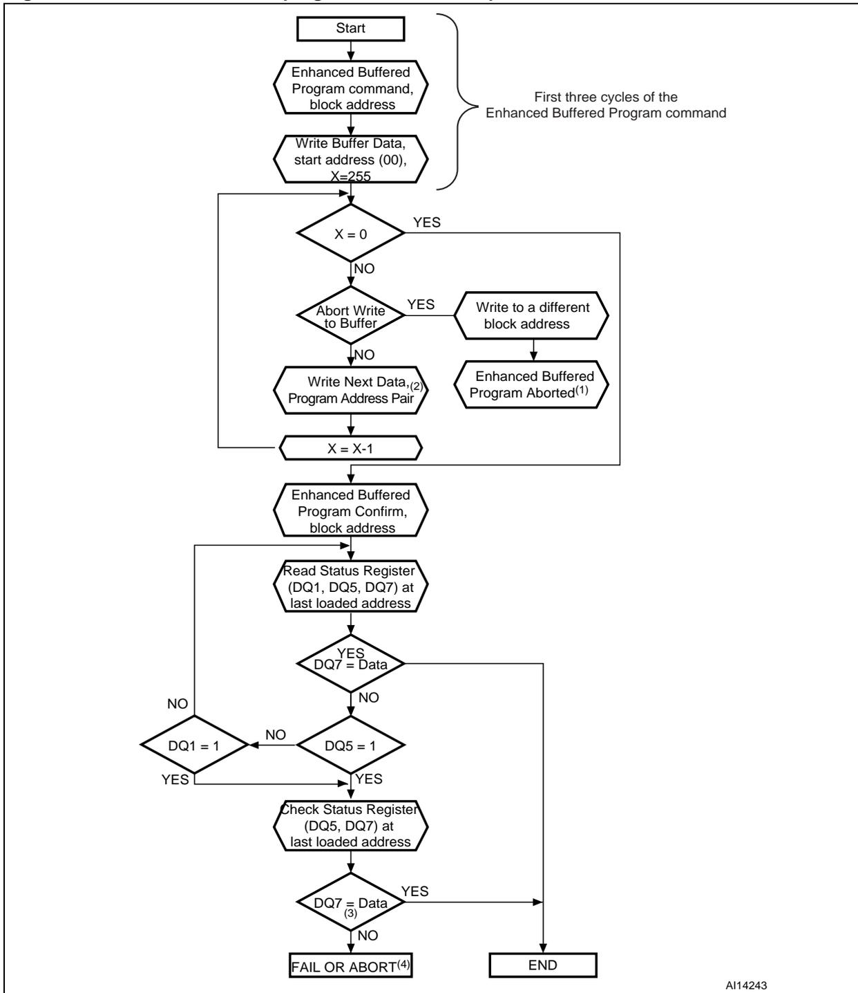
1. A buffered program abort and reset must be issued to return the device in read mode.
