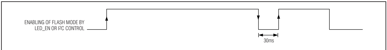
Figure 3. Flash Safety Timer Reset Inhibit Period
