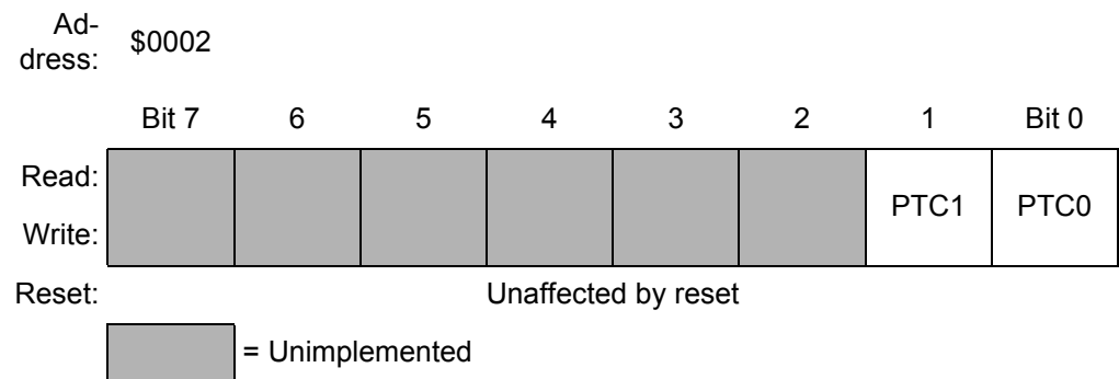
Figure 14-8. Port C Data Register (PTC)
