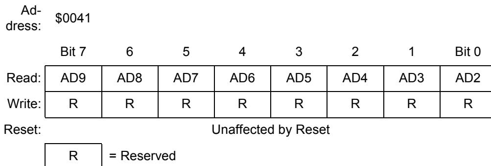
Figure 18-4. ADC Data Register High (ADRH) Left Justified Mode
