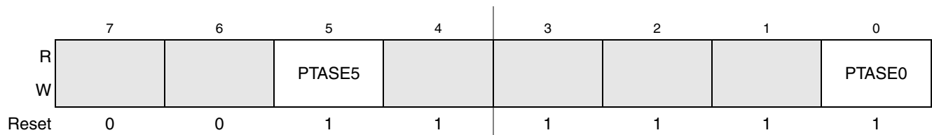
Figure 6-5. Output Slew Rate Control Enable for Port A (PTASE)
