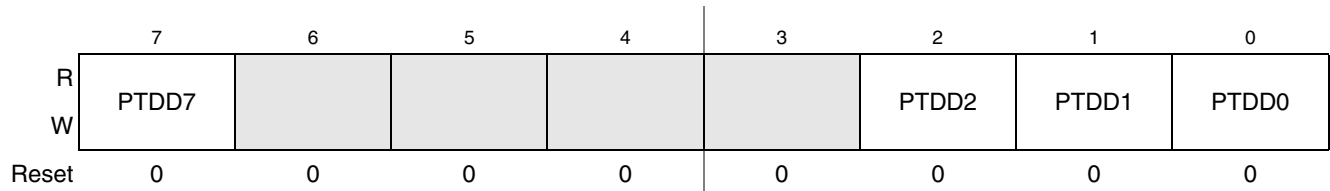
Figure 6-17. Port D Data Register (PTDD)
