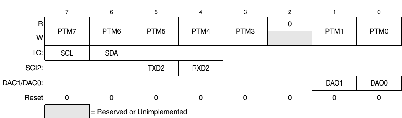
Figure 3-10. Port M I/O Register (PTM)
