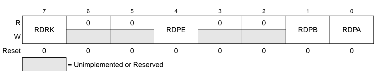
Figure 21-15. Reduced Drive Register (RDRIV)
