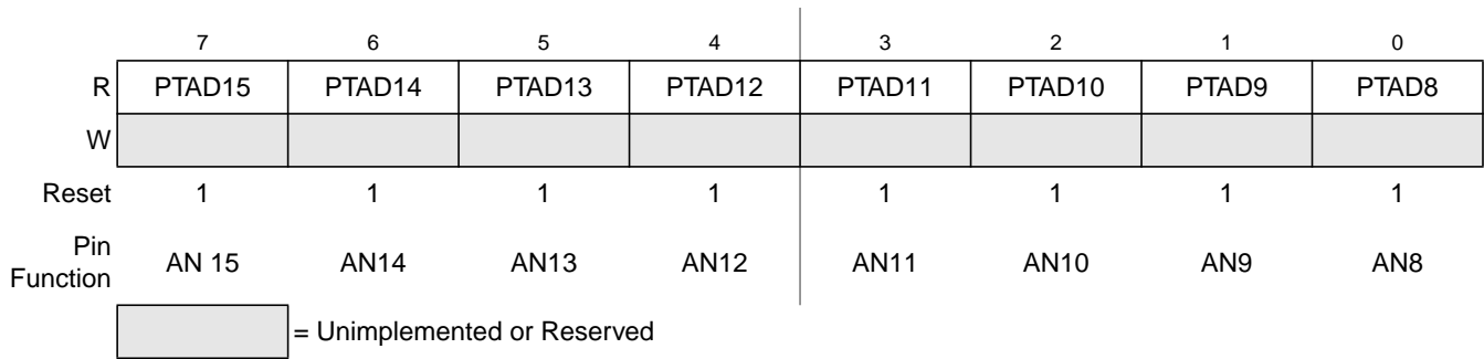
Figure 7-16. Port Data Register 0 (PORTAD0)
