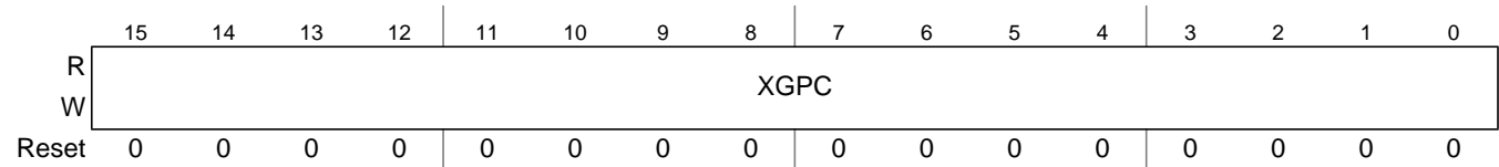
Figure 5-10. XGATE Program Counter Register (XGPC)
