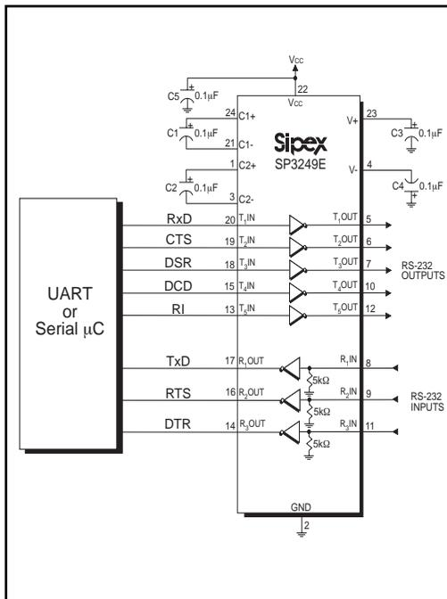
Figure 6. Interface Circuitry Controlled by Microprocessor Supervisory Circuit
