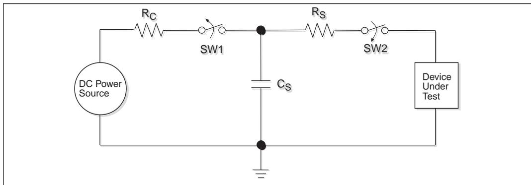
Figure 16. ESD Test Circuit for Human Body Model
