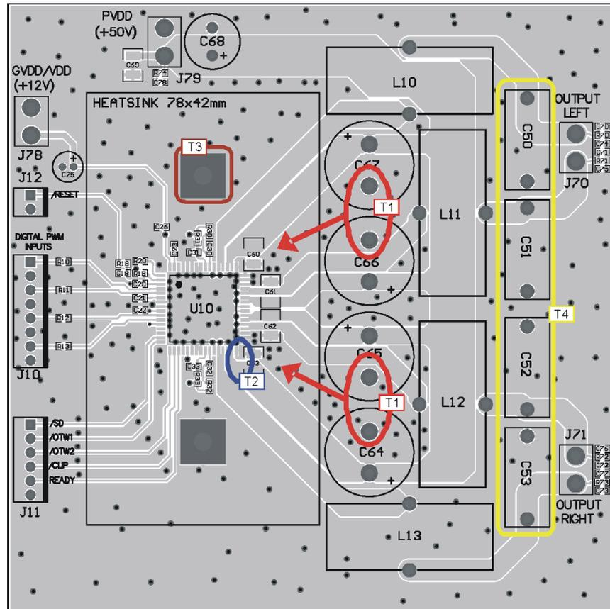
**Note T1:** PVDD decoupling bulk capacitors C60-C64 should be as close as possible to the PVDD and GND\_X pins, the heat sink sets the distance. Wide traces should be routed on the top layer with direct connection to the pins and without going through vias. No vias or traces should be blocking the current path.
