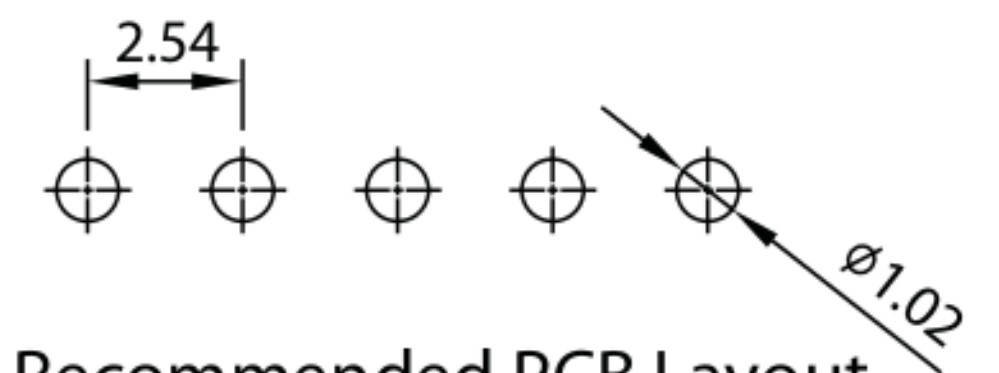
Recommended PCB Layout (PCB TOLERANCE \pm 0.05 )
