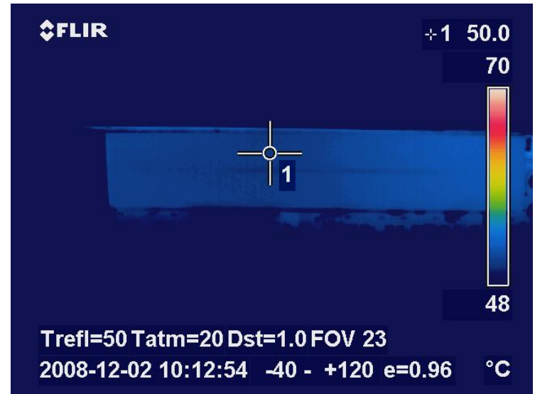
Thermal temp. of surface of heat sink (Blower is under operation)
