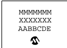
8-Lead SOIC (208 mil)
