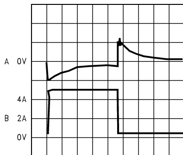
Load Transient Response for Continuous Mode V_{IN} = 20V, V_{OUT} = 5V L = 10 \mu H, C_{OUT} = 400 \mu F, C_{OUT}ESR = 13 m\Omega
