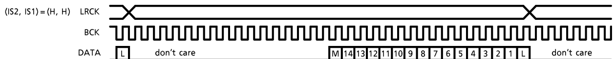
Figure 1d Data Input Format Example 4 ((IS2, IS1) = (H, H); effective data before the change point of LRCK, 16bit/ch)
