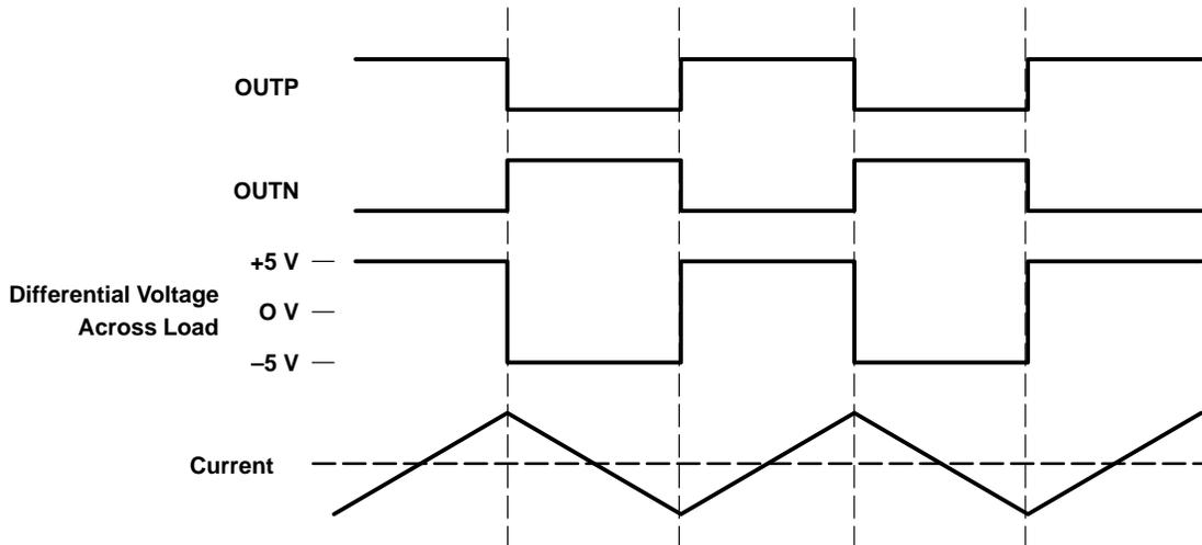
**Figure 10. Traditional Class-D Modulation Scheme Output Voltage and Current Waveforms Into an Inductive Load With No Input**
