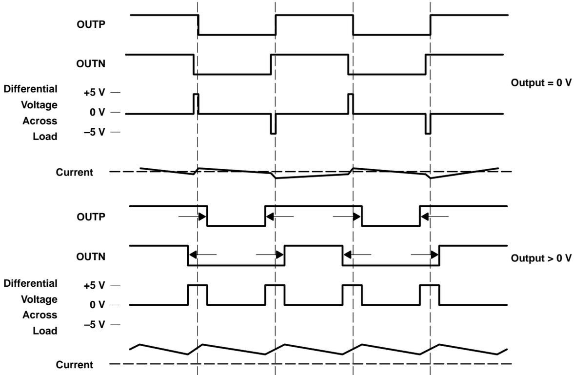
Figure 11. The TPA2000D1 Output Voltage and Current Waveforms Into an Inductive Load
