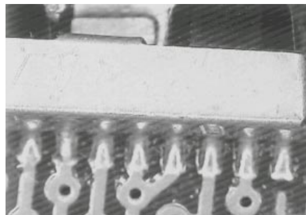
Picture 4. Unit self-aligns after reflow.
